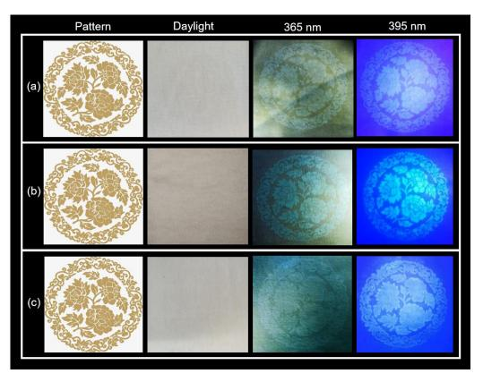
**Figure 5.** Anti-counterfeit patterns were designed and printed on cotton fabric under illumination at 365 nm and 395 nm. The C-dots were prepared using (**a**) Indigo, (**b**) *Carcuma longa*, and (**c**) *Sophora japonica* L.
