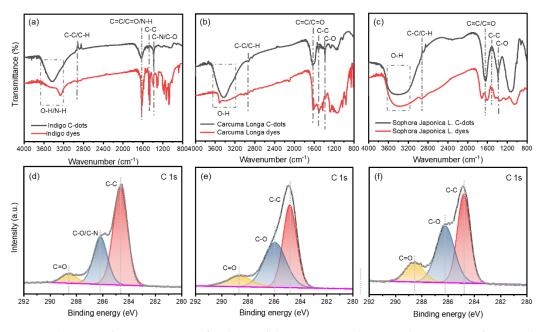
**Figure 3.** (**a**–**c**) are the FT-IR spectra of C-dots and dyes, corresponding to Indigo, *Carcuma longa*, and *Sophora japonica* L., respectively; (**d**–**f**) are high-resolution XPS C 1 s spectra corresponding to C-dots derived from Indigo (**d**), *Carcuma longa* (**e**), and *Sophora japonica* L. (**f**).
