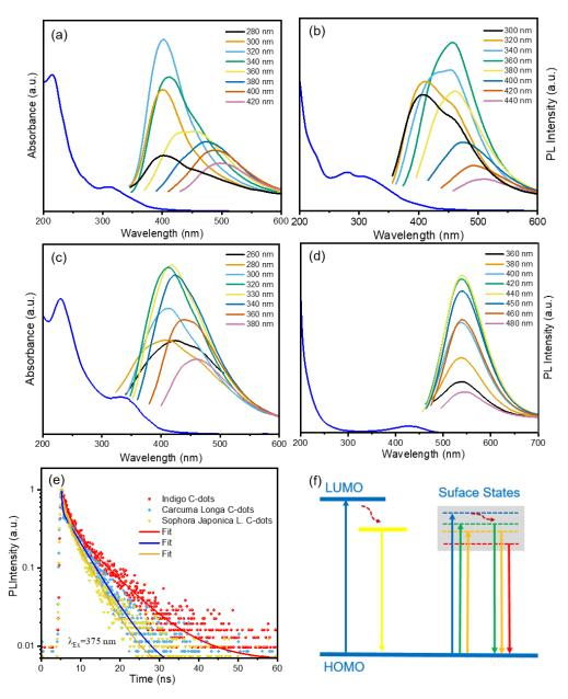
**Figure 4.** UV-Vis absorption and PL spectra of the C-dots dispersed in water using precursors of (a) Indigo, (b) *Carcuma longa*, and (c) *Sophora japonica* L.; (d) Absorption and PL spectra of the *Carcuma longa* dyes; (e) PL decay curves of the C-dots dispersed in water; (f) Possible electronic band structure for *Carcuma longa* dyes (left) and the C-dots (right).
