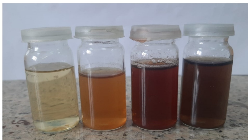
Figure 2. Green synthesised copper nanoparticles and colour change with an increase in the reduction time.
