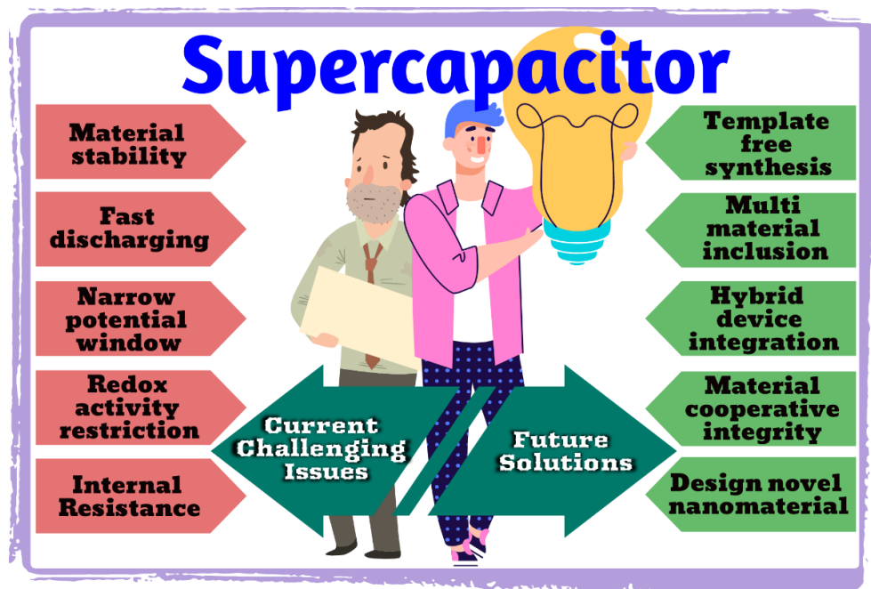
Figure 14. Schematic of several current challenges and future solutions to obtaining highly applicable supercapacitor devices.
