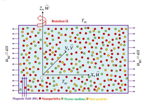
Figure 1. Schematic flow configuration.
