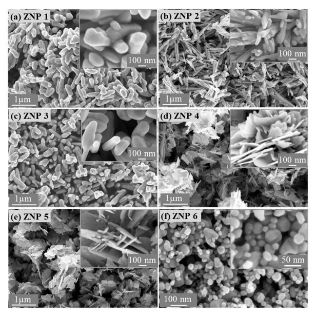
**Figure 1.** Field emission scanning electron microscope images of the ZnO samples: (a) ZNP 1 (annealing, 700  $^{\circ}$ C, 10 h), (b) ZNP 2 (annealing, 400  $^{\circ}$ C, 10 h), (c) ZNP 3 (annealing, 700  $^{\circ}$ C, 6 h), (d) ZNP 4 (precipitation, [NaOH] = 0.4 M), (e) ZNP 5 (precipitation, [NaOH] = 0.7 M), and (f) ZNP 6 (microwave-assisted synthesis).
