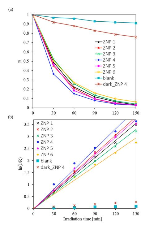
**Figure 4.** RhB degradation under UV-Vis light irradiation: (**a**) R ( $C/C_0$ ) values of RhB and (**b**) the ln(1/R) as a function of irradiation time.
