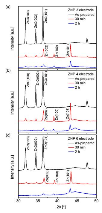
**Figure 5.** XRD patterns of the electrodes with three nanostructures: (a) nanorod (ZNP 3), (b) lamellar (ZNP 4), and (c) nanoparticle (ZNP 6) after different reduction time (as-prepared, after 30 min of reduction, and after 2 h of reduction at -1.0 V vs. RHE).
