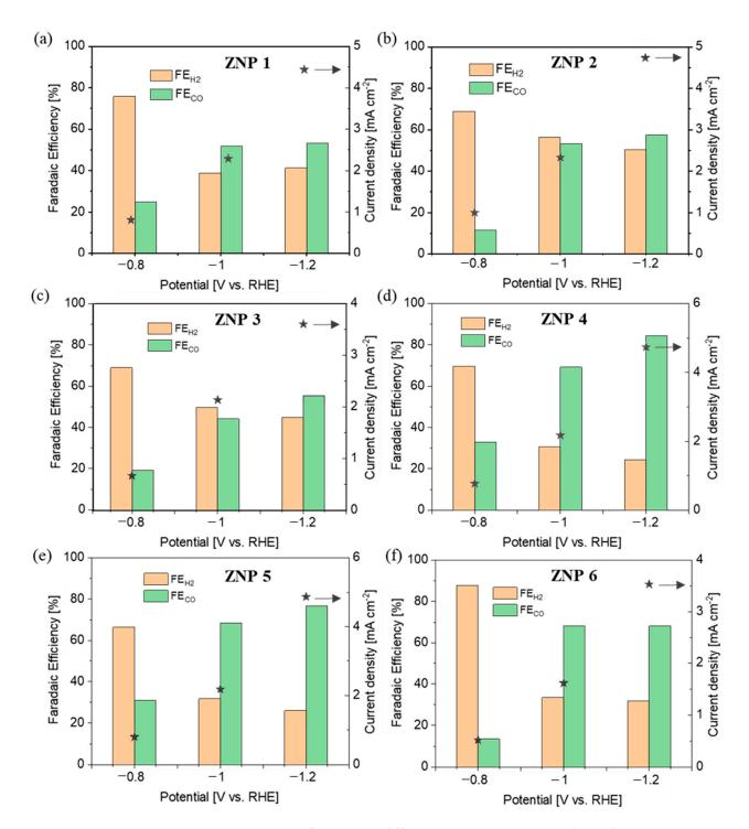
**Figure 7.** CO<sub>2</sub>RR performance at different potentials on various electrodes: (a) ZNP 1, (b) ZNP 2, (c) ZNP 31, (d) ZNP 4, (e) ZNP 5, and (f) ZPN 6.
