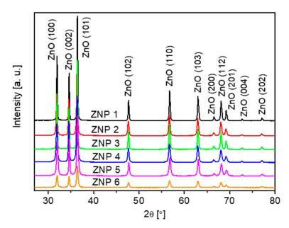
**Figure 2.** XRD patterns of the ZnO samples: ZNP 1 (annealing, 700  $^{\circ}$ C, 10 h), ZNP 2 (annealing, 400  $^{\circ}$ C, 10 h), ZNP 3 (annealing, 700  $^{\circ}$ C, 6 h), ZNP 4 (precipitation, [NaOH] = 0.4 M), ZNP 5 (precipitation, [NaOH] = 0.7 M), and ZNP 6 (microwave-assisted synthesis).
