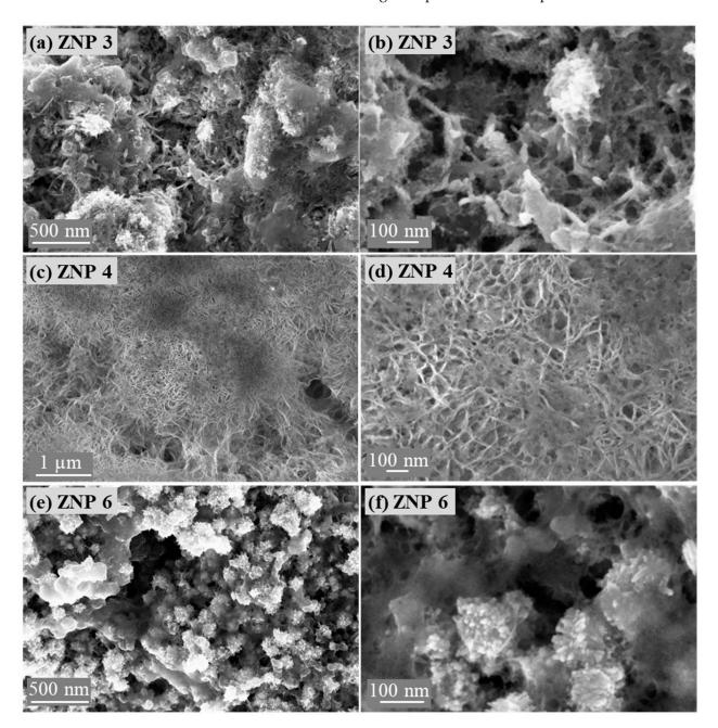
**Figure 6.** Field emission scanning electron microscope images of the reduced electrodes: **(a,b)** ZNP 3, **(c,d)** ZNP 4, and **(e,f)** ZNP 6.
