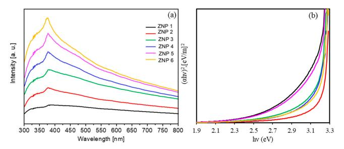
Figure 3. (a) Optical density spectra of all ZnO samples; (b) Tauc's plot for energy bad gap determination.
