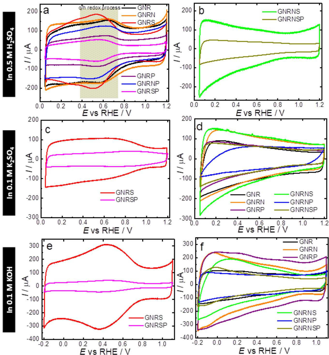
**Figure 3.** CV obtained for the GC electrodes modified with  $150 \mu\text{g cm}^{-2}$  of undoped or doped GNR applied in  $\text{N}_2$ -saturated  $0.5 \text{ M H}_2\text{SO}_4$ ,  $0.1 \text{ M K}_2\text{SO}_4$ , and  $0.1 \text{ M KOH}$ . Potential scan rate:  $50 \text{ mV s}^{-1}$  (scans were initiated at  $1.2 \text{ V}$ ).
