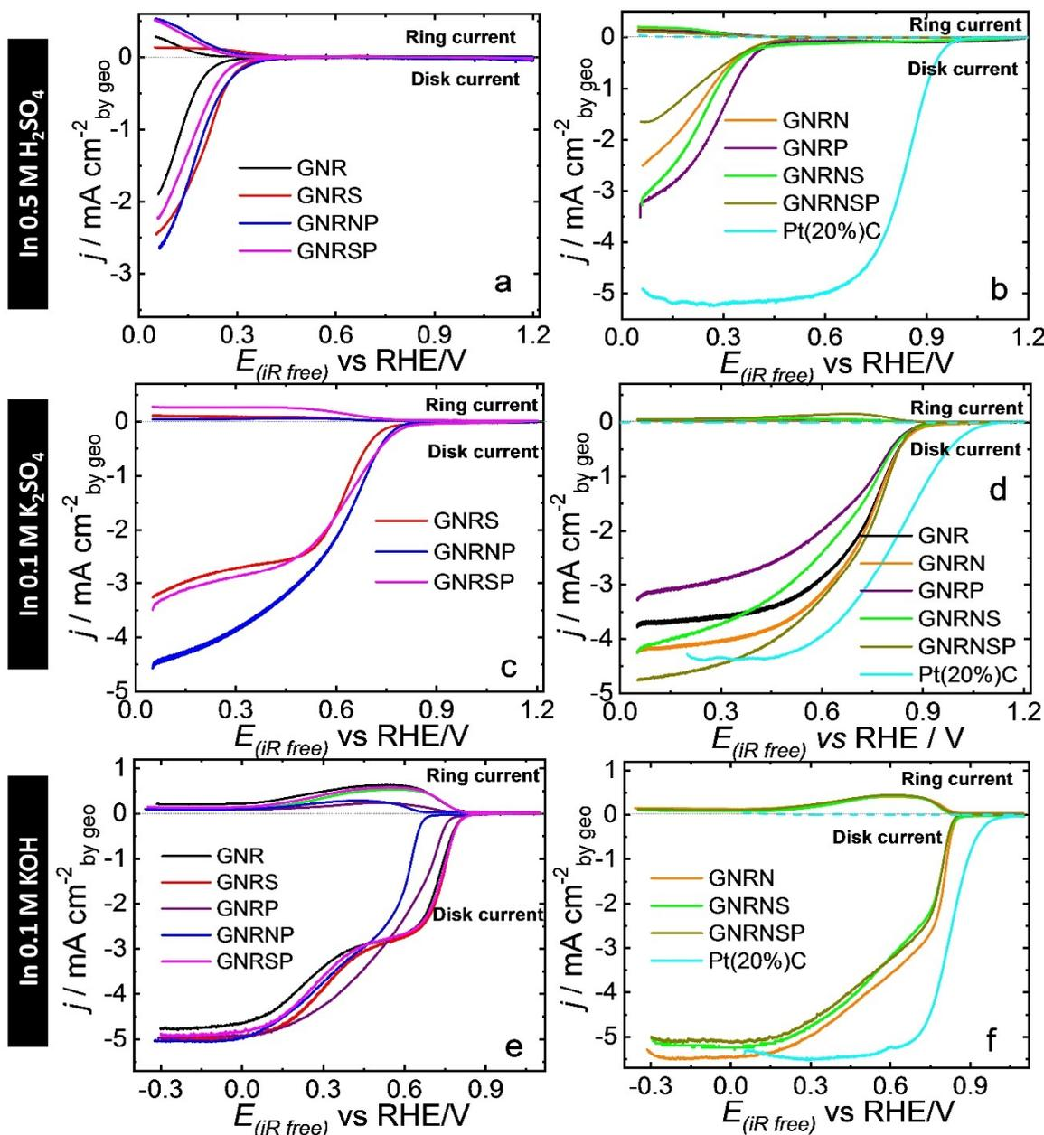
**Figure 4.** Results obtained from the LSV analysis conducted in a RRDE system for GC modified with  $150 \mu\text{g cm}^{-2}$  of undoped or doped GNR catalysts under the following conditions: scanning at the potential of  $10 \text{ mV s}^{-1}$ ; RRDE rotation at 1600 rpm; electrolyte solutions applied:  $\text{O}_2^-$  saturated  $0.5 \text{ M H}_2\text{SO}_4$ ,  $0.1 \text{ M K}_2\text{SO}_4$ , and  $0.1 \text{ M KOH}$  (scans were initiated at 0.05 or  $-0.3 \text{ V}$ ).
