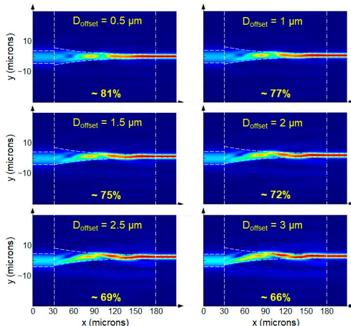
**Figure A1.** Simulated electric field distributions and corresponding transmittances of designed tapered fibers for different lateral offsets ( $D_{\text{offset}}$ ) ranging from 0.5 to 3  $\mu\text{m}$ .
