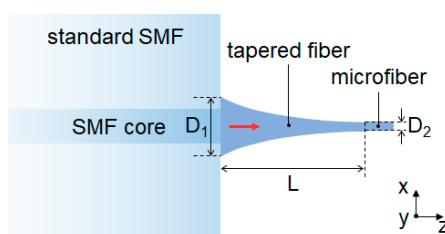
**Figure 1.** Schematic of the tapered fiber on a cleaved standard SMF tip. A nonlinear tapered fiber was designed to direct the guided light from a standard SMF into a microfiber. The cartesian coordinate is shown with its  $z$ -direction along the optical axis of optical fiber.
