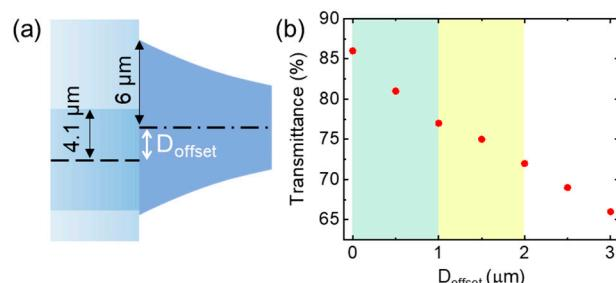
**Figure 3.** (a) Schematic of the lateral offset (denoted with  $D_{\text{offset}}$ ) between the SMF and taper structure. (b) Calculated transmittance as a function of the lateral offset ( $D_{\text{offset}}$ ).
