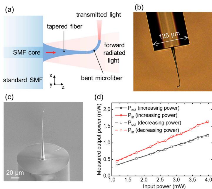
**Figure 4.** (a) Schematic of the fabricated structure. The transition structure included a nonlinear tapered fiber ( $L = 150\text{ }\mu\text{m}$ ,  $D_1 = 12\text{ }\mu\text{m}$ ,  $D_2 = 1\text{ }\mu\text{m}$ ) and a circular  $90^\circ$  bent microfiber with a bending radius of  $12\text{ }\mu\text{m}$ . (b) Microscopic and (c) SEM images of the fabricated sample. (d) Measured output power as a function of the input laser power for the fabricated sample.
