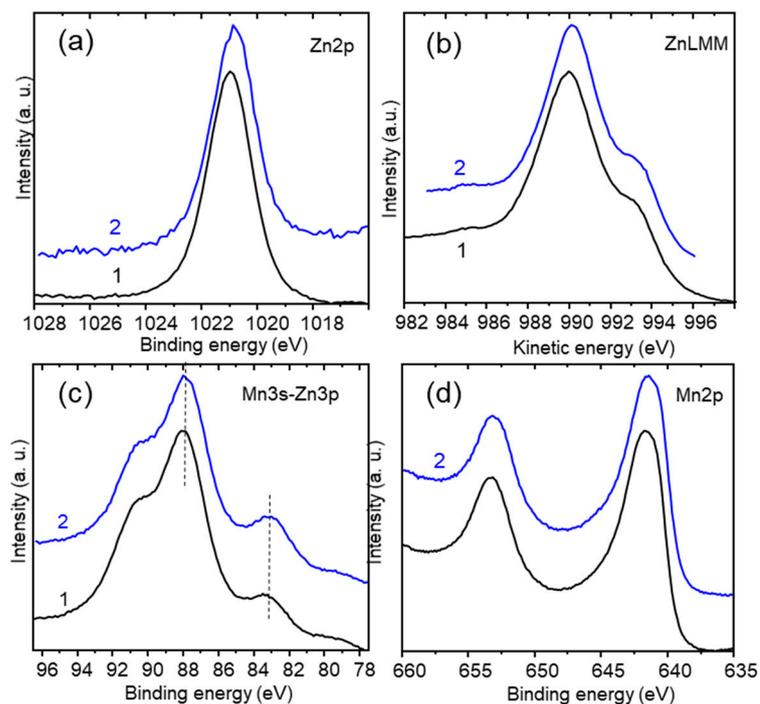
**Figure 15.** XPS of electrode of SCC PVP-LiClO<sub>4</sub>: (a) Zn2p, (b) ZnLMM, (c) M3s Zn3p, (d) Mn2p. Electrodes: (1) as-deposited, (2) after 300 CV cycles finishing under reducing conditions.
