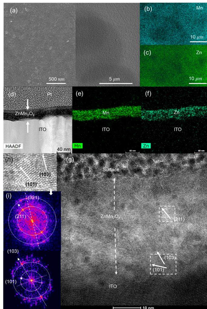
**Figure 3.** As-deposited  $\text{ZnMn}_2\text{O}_4$  electrode: (a) SEM, (b) Mn, (c) Zn EDS images of the electrode surface; (d) HAADF; (e) Zn and (f) Mn EDS images of the electrode cross-section; (g) HRTEM image of the cross-section; (h) magnification of the marked zone; (i) FFTs of the film cross-section.
