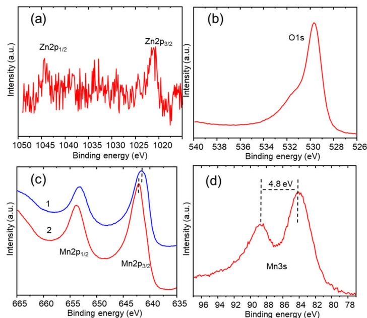
**Figure 7.** XPS spectra of (a) Zn2p, (b) O1s, (c) Mn2p, (d) Zn3p-Mn3s of the ZnMn<sub>2</sub>O<sub>4</sub> electrode after 3000 CV cycles.
