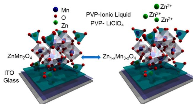
**Figure 12.** Scheme of the transformation from ZnMn<sub>2</sub>O<sub>4</sub> to Zn<sub>1-x</sub>Mn<sub>3-x</sub>O<sub>4</sub>.
