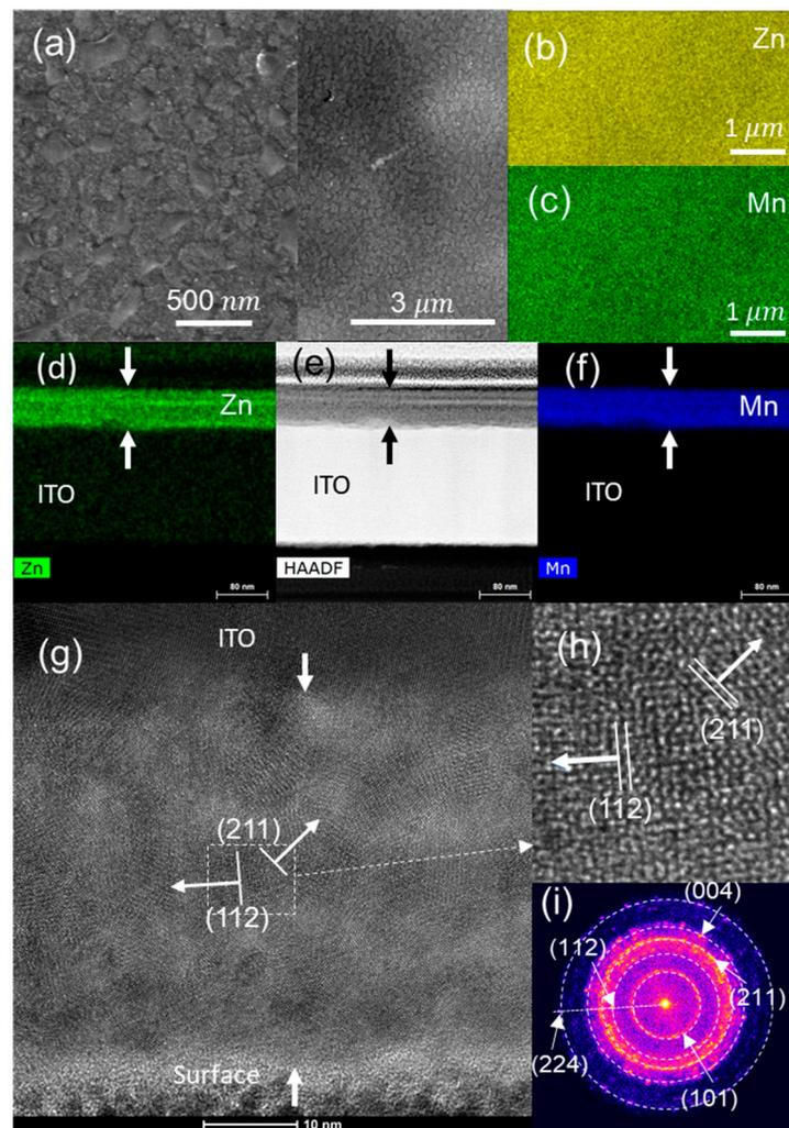
**Figure 10.** SCC with PVP-ionic liquid as electrolyte after 300 CV cycles: (a) SEM; (b) Zn and (c) Mn EDS images of the surface of the electrode; (d) Zn and (f) Mn EDS images; (e) HAADF images of the electrode cross-section; (g) HRTEM image of the cross-section; (h) magnification of the marked zone; (i) FFT of the film cross-section.
