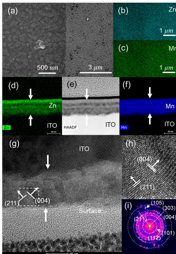
**Figure 14.** SCC with PVP-LiClO<sub>4</sub> as electrolyte after 300 CV cycles: (a) SEM; (b) Zn and (c) Mn EDS images of the surface of the electrode; (d) Zn and (f) Mn EDS images; (e) HAADF images of the electrode cross-section; (g) HRTEM image of the cross-section; (h) magnification of the marked zone; (i) FFT of the film cross-section.
