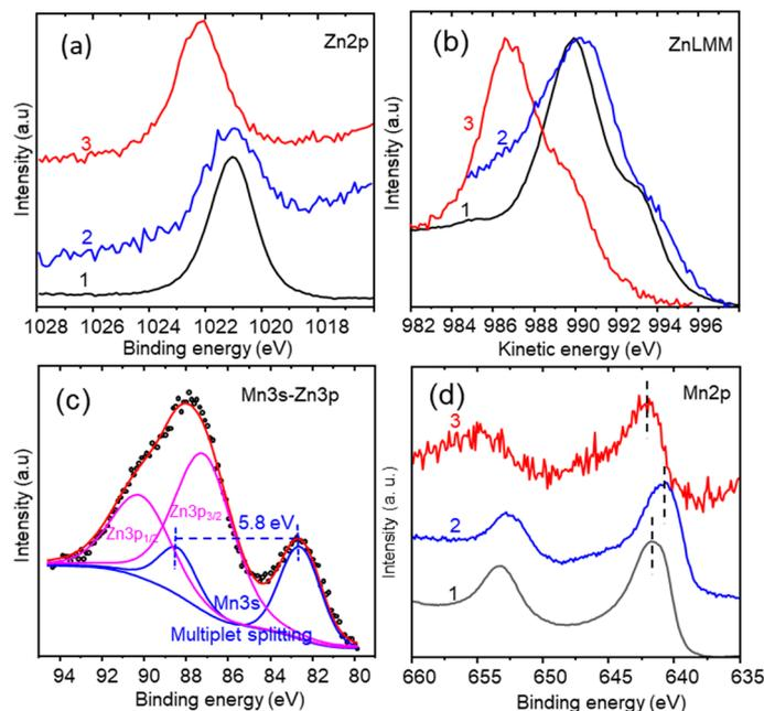
**Figure 11.** XPS of electrode of SCC PVP-Ionic Liquid: (a) Zn2p, (b) ZnLMM, (c) M3s Zn3p, (d) Mn2p. Electrodes: (1) as-deposited, (2) after 300 CV cycles finishing under reducing conditions, (3) after 300 cycles of CV finishing under oxidizing condition.
