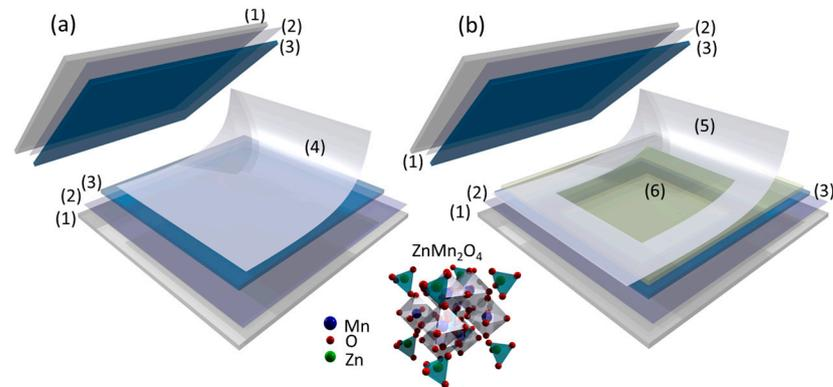
**Figure 1.** Scheme of the symmetric supercapacitors (a) using an acetate membrane soaked in 1.0 M  $\text{Na}_2\text{SO}_4$  aqueous solution, and (b) with a Meltonix separation polymer and electrolyte formed by PVP- ionic liquid or PVP-  $\text{LiClO}_4$ . (1) Glass, (2) ITO, (3)  $\text{ZnMn}_2\text{O}_4$ , (4) acetate membrane soaked with 1.0 M  $\text{Na}_2\text{SO}_4$ , (5) separation polymer (frame), (6) non-aqueous electrolyte (PVP-ionic liquid or PVP- $\text{LiClO}_4$ ).
