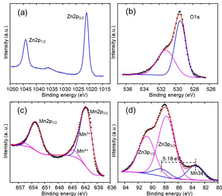
**Figure 4.** XPS spectra of (a) Zn2p, (b) O1s, (c) Mn2p, (d) Zn3p-Mn3s of the as-deposited  $ZnMn_2O_4$  electrode.
