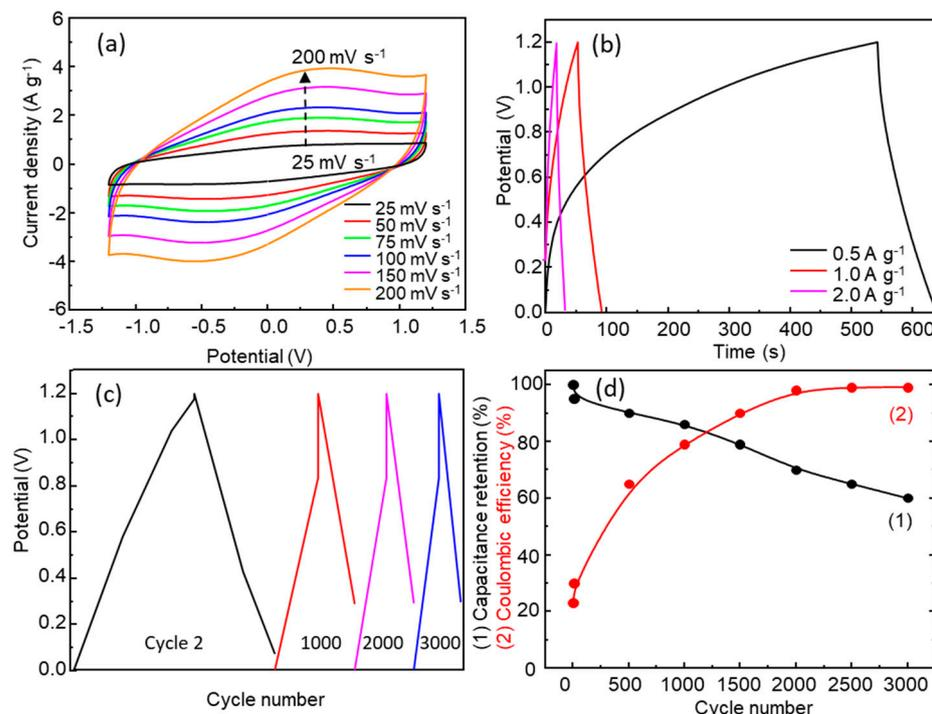
**Figure 13.** SCC with PVP-LiClO<sub>4</sub>: (a) CV cycles with a  $\pm 1.2$  V potential window at scan rates from 25 to  $200 \text{ mV s}^{-1}$ ; (b) GCD at current densities of  $0.5 \text{ A g}^{-1}$ ,  $1.0 \text{ A g}^{-1}$ ,  $2.0 \text{ A g}^{-1}$ ; (c) GCD cycles 2, 1000, 2000, and 3000; (d) capacitance retention and Coulombic efficiency (GCD cycles).
