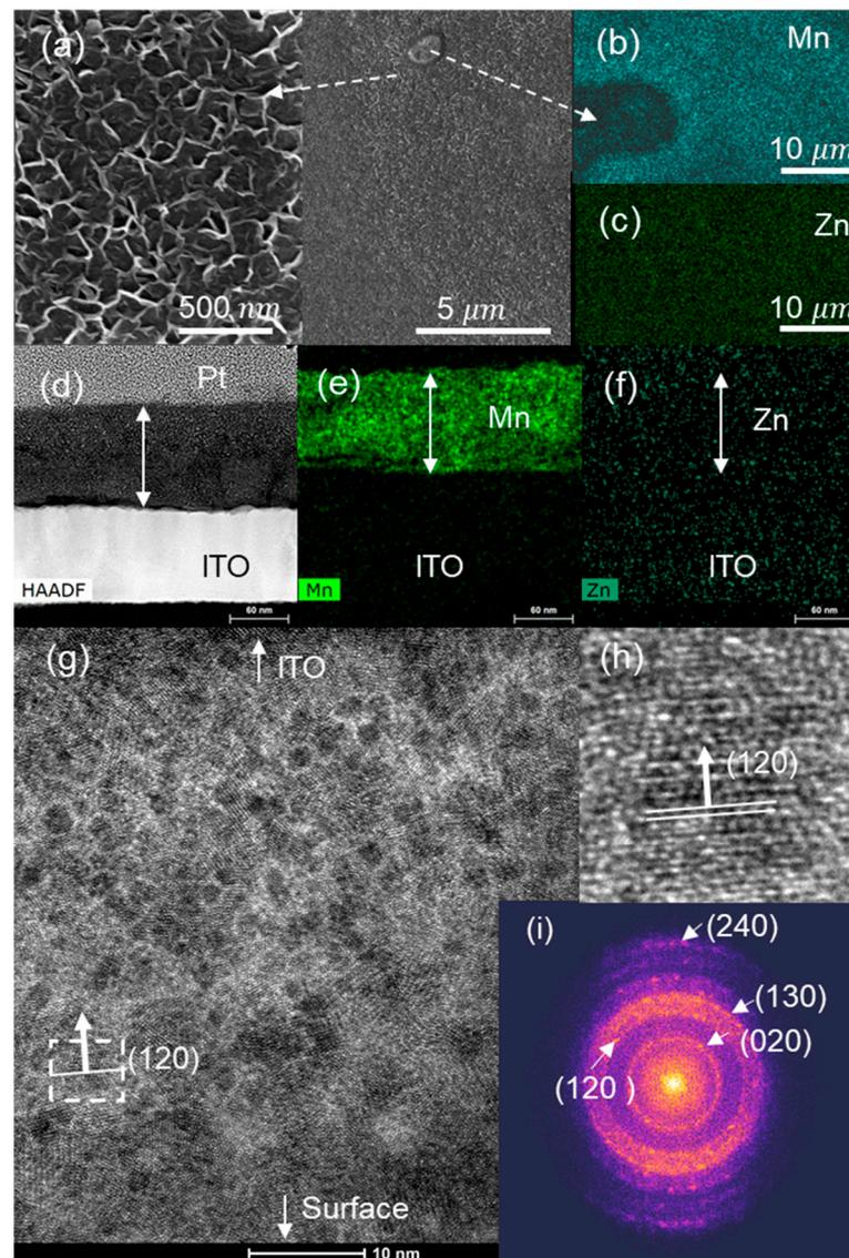
**Figure 6.** ZnMn<sub>2</sub>O<sub>4</sub> electrode after 300 CV cycles: (a) SEM; (b) Mn and (c) Zn EDS images of the electrode surface; (d) HAADF; (e) Mn and (f) Zn EDS images of the electrode cross-section; (g) HRTEM image of the cross-section, (h) magnification of the marked zone; (i) FFTs of the film cross-section.
