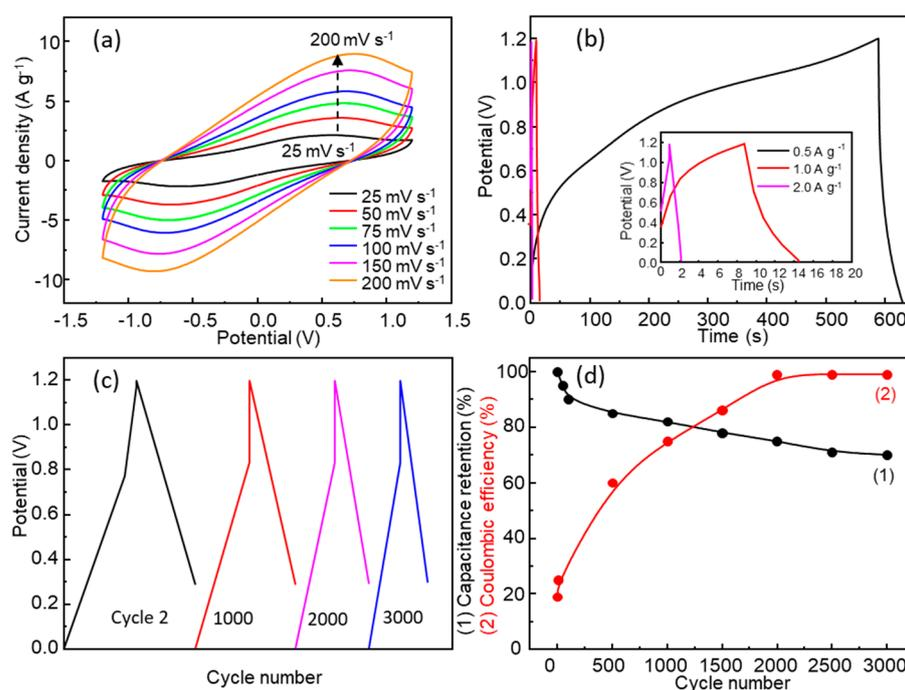
**Figure 9.** SCC with PVP-Ionic liquid: (a) CV cycles with a  $\pm 1.2 \text{ V}$  potential window at scan rates from 25 to  $200 \text{ mV s}^{-1}$ ; (b) GCD at current densities of  $0.5 \text{ A g}^{-1}$ ,  $1.0 \text{ A g}^{-1}$ ,  $2.0 \text{ A g}^{-1}$ ; (c) GCD cycles 2, 1000, 2000, and 3000; (d) capacitance retention and Coulombic efficiency (GCD cycles).
