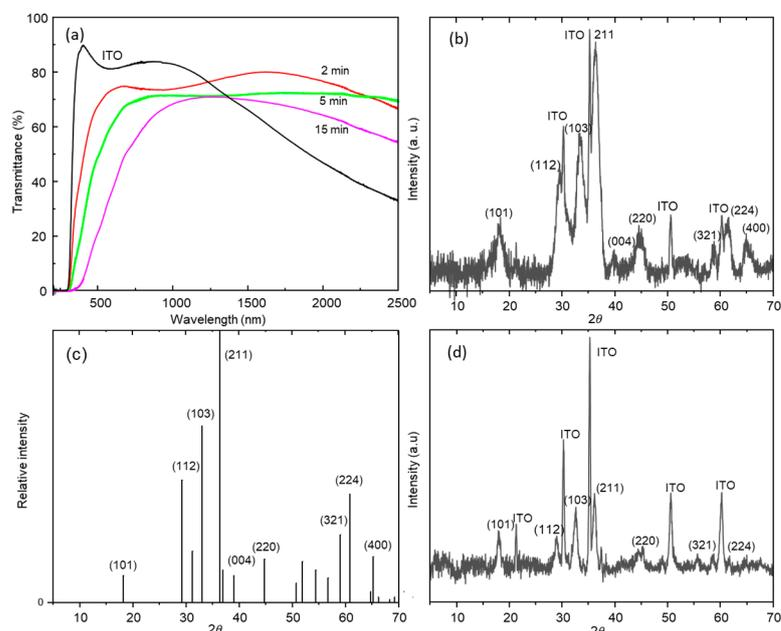
**Figure 2.** (a) Optical transmittance spectra of the  $\text{ZnMn}_2\text{O}_4$ /ITO/glass electrodes at different deposition times; (b) XRD pattern of the as-deposited electrode of  $\text{ZnMn}_2\text{O}_4$  on ITO corresponding to deposition time of 15 min, (c) XRD standard diffraction pattern of  $\text{ZnMn}_2\text{O}_4$  PDF 01-071-2499, (d) 5 min.
