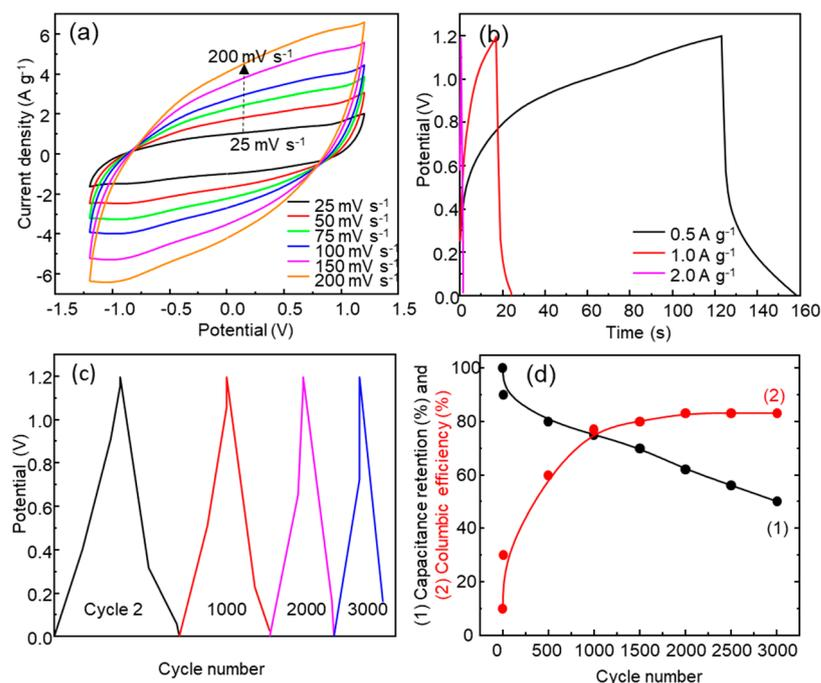
**Figure 8.** (a) Cyclic voltammetry curves with  $\pm 1.2$  V potential window at scan rates from 25 to 200  $\text{mV s}^{-1}$ ; (b) GCD at different current densities of 0.5  $\text{A g}^{-1}$ , 1.0  $\text{A g}^{-1}$ , and 2.0  $\text{A g}^{-1}$ ; (c) GCD at cycle 2, 1000, 2000, and 3000; (d) capacitance retention and Coulombic efficiency (GCD cycles) for the SSC 1.0 M  $\text{Na}_2\text{SO}_4$ .
