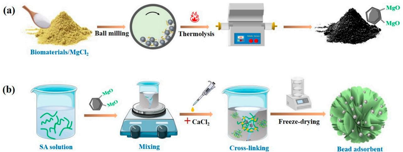
**Figure 1.** Schematic diagrams for the (a) MgBC and (b) bead preparation.
