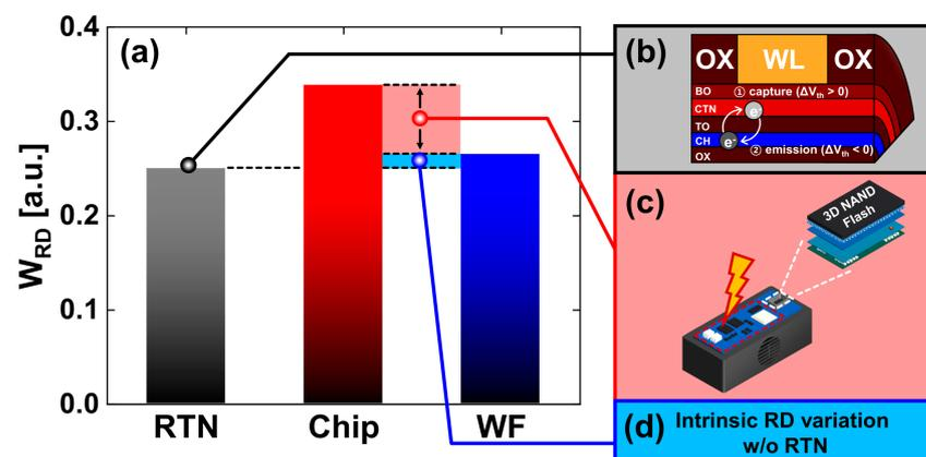
**Figure 3.** (a) Distribution width of read variation in chip and WF obtained by reading iteratively seven days after completion of programming. (b) RTN behavior with charge capture and emission. (c) Noise from the peripheral circuitry in the chip–level equipment. (d) Measured intrinsic read variation in WF except for RTN.
