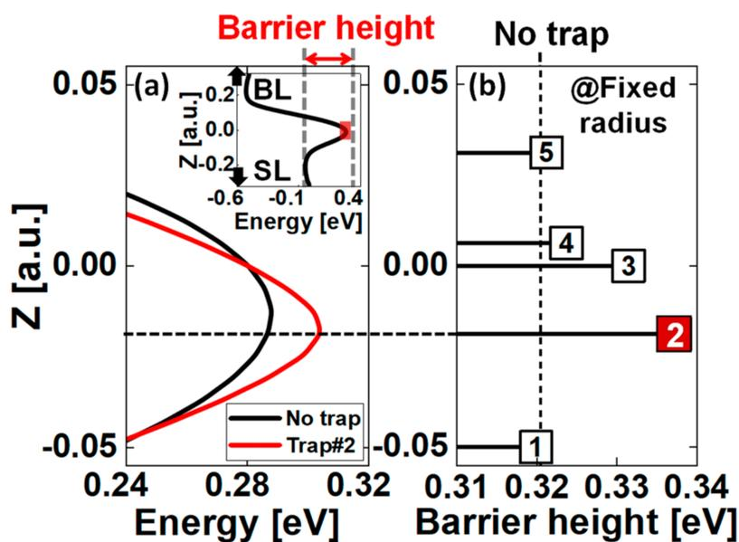
**Figure 7.** (a) Band diagram of a channel enlarged by the channel length of the target cell in an inset, with and without a single trap (or before and after programming) at trap #2 in (b), (b) change in barrier height with respect to the position of single trap numbered from 1 to 5.
