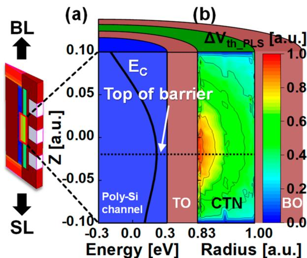
**Figure 6.** (a) Band diagram of the poly-Si channel in the read operation after PGM operation and (b) contour plot with the magnitude of  $\Delta V_{th\_PLS}$  highlighted in different colors at different nitride traps in a target cell in the string.
