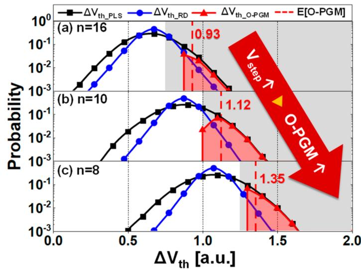
**Figure 4.**  $\Delta V_{th\_PLS}$  distribution (black lines) from  $(n - 1)$ th programming pulse to  $n$ th programming pulse during the ISPP,  $\Delta V_{th\_RD}$  by read variation (blue lines),  $\Delta V_{th\_O-PGM}$  by O-PGM (red lines), and the conditional expected values of O-PGM (red dashed lines) to (a)  $V_{step} = 0.75$  a.u., (b)  $V_{step} = 1$  a.u., and (c)  $V_{step} = 1.25$  a.u., respectively; grey regions represent abnormal program cell regimes.
