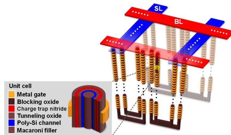
**Figure 1.** Schematic of a 3D U-shaped SMArT structure (inset: a nanowire thin film transistor cell composed of multiple materials based on charge trap nitride as storage layer). The channel strings are connected to the sourceline (SL) and the bitline (BL), which are the source of electrons, and a signal line connected to the page buffer, which is a circuit that converts the analog channel current into digital data (bits), respectively.
