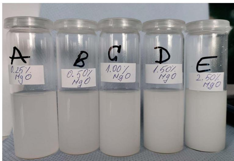
Figure 1. Samples: MgO nanocolloids with PEG 400.
