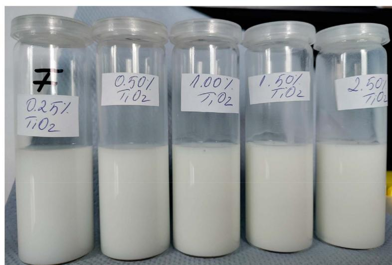
Figure 2. Samples: TiO<sub>2</sub> nanocolloids with PEG 400.
