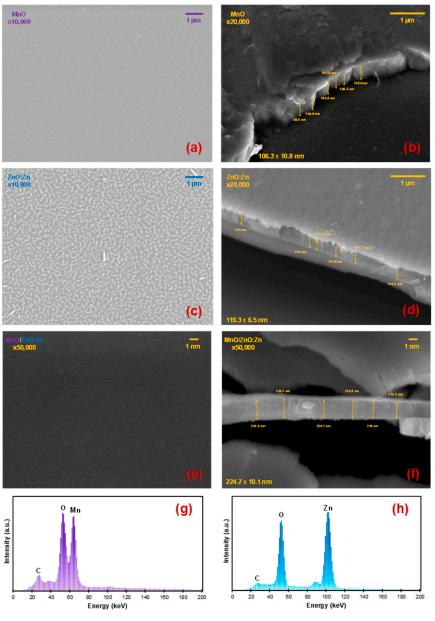
**Figure 5.** (a) SEM micrograph of surface of MnO (MnGl) at  $\times 10,000$ , (b) cross-sectional image of MnO at  $\times 20,000$ , (c) micrograph of surface of ZnO:Zn (ZnGl), (d) cross-sectional image of ZnO:Zn at  $\times 20,000$ , (e) micrograph of surface of structure MnO/ZnO:Zn at  $\times 50,000$ , (f) cross-sectional image of structure MnO/ZnO:Zn at  $\times 50,000$ , (g) EDS analysis of MnGl, (h) EDS analysis of ZnGl.
