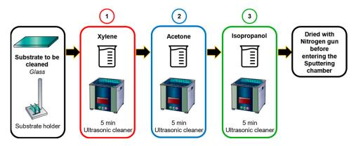
**Figure 1.** Substrate cleaning process before sputtering deposition.
