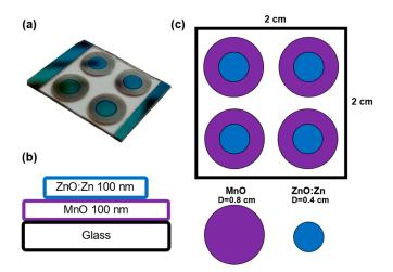
**Figure 2.** (a) Photograph of complete MnO/ZnO heterostructure, (b) cross-sectional diagram of structure, indicating thickness of as-prepared films, (c) area of deposition showing stainless-steel mask to define each material.
