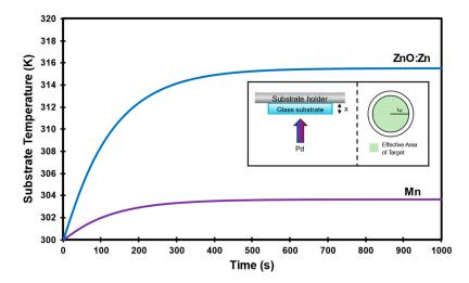
**Figure 6.** Solution of 1D heat equation for glass substrate for Mn and ZnO:Zn deposition. Stabilization time of deposition is around 500 s according to equation. Inset shows graphical model used in assumptions and effective area of a target.
