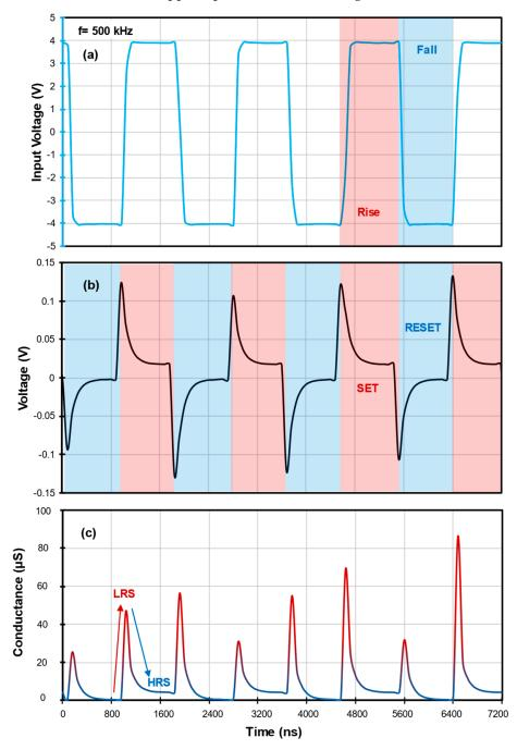
**Figure 8.** Applying a  $\pm 4\mathrm{V}$  square signal to MnO/ZnO:Zn structure, we obtain (a) input signal with rise and fall signals indicated in red and blue, respectively; (b) response of structure as pulses, where the switching speed is measured in oscilloscope and indicated as  $17 \pm 0.82$  ns for HRS to LRS and  $439 \pm 21.9$  ns for LRS to HRS; and (c) conductance for applied pulses where switching ratio is calculated as  $2.11 \times 10^4 \pm 6.59 \times 10^4$ .
