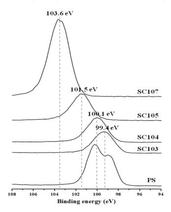
**Figure 5.** Si-2p XPS profiles of PS and SiO<sub>x</sub>-CNT samples.
