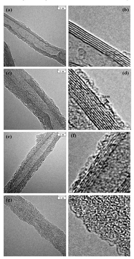
Figure 3. TEM images of (a,b) pristine CNTs, (c,d) SC103, (e,f) SC104, (g,h) SC107.
