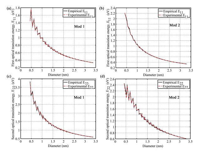
**Figure 2.** Plot of absolute deviations (errors) of first  $(E_{11})$  and second  $(E_{22})$  optical transition energy vs. nanotube diameter  $(d_t)$ . (a) Absolute deviations of empirical  $E_{11}$  from experimental data for both mod 1 and mod 2; (b) Absolute deviations of empirical  $E_{22}$  from experimental data for both mod 1 and mod 2.
