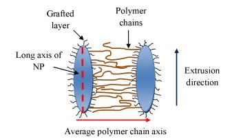
**Figure 10.** A schematic representation of the relative orientations of NPs and PA6 chains in nanocomposites.
