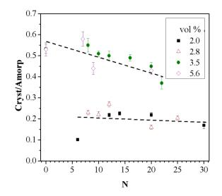
**Figure 7.** Total crystalline/amorphous ratio variation with respect to the processing parameter *N* at the indicated NP compositions. Lines are drawn as a visual guide.
