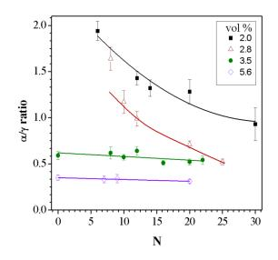
**Figure 6.** Variation of  $\alpha/\gamma$  crystalline ratios with the processing parameter *N* for samples at the indicated NP compositions. The solid lines are drawn as a guideline for the eye.
