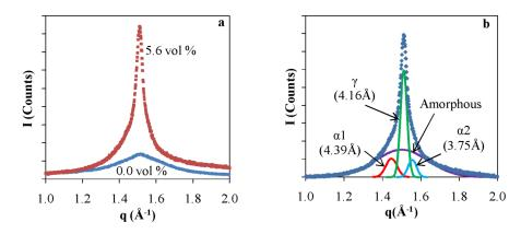
Figure 5. (a) Powder X-ray patterns of extruded PA6 with and without NPs at N = 0; and (b) Peak deconvolution of X-ray data for 5.6 vol % nanocomposite.
