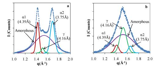
Figure 4. X-ray patterns and analysis of Poly Amide 6 (PA6) films (a) Pristine; and (b) Chaotically blended at N = 30.
