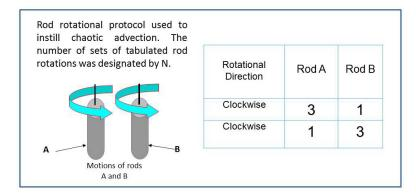
Figure 2. Schematic presentation of the agitator in chaotic advection and the time evolution of the slow. The agitation scheme used in the current study for N = 1 is presented.
