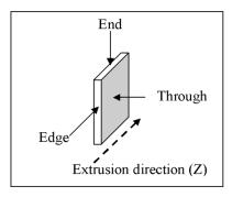
Figure 3. Directions of incident X-ray beams with respect to the extrusion direction. X and Y define the plane of the film and Z corresponds to the extrusion directions.
