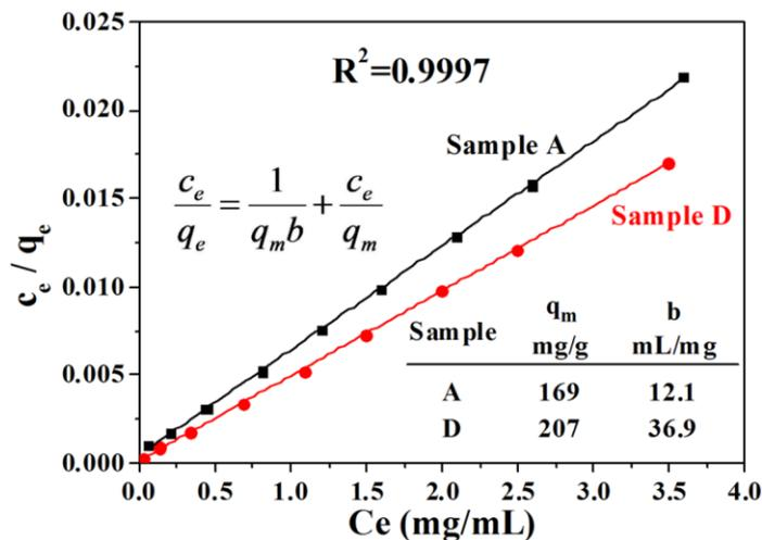
**Figure 6.** The Hb protein adsorption properties of Sample A (pH 5) and Sample D (pH 11). The linear relationship between  $c_e/q_e$  and  $c_e$ .
