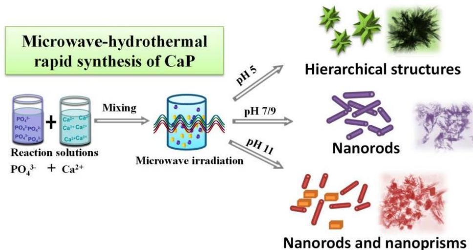
**Figure 4.** Schematic illustration for the synthesis of calcium phosphate nanostructures with the microwave-assisted hydrothermal method under different pH values.
