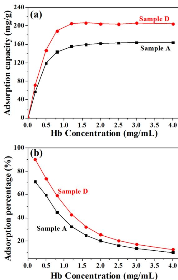
**Figure 5.** The Hb protein adsorption properties of Sample A (pH 5) and Sample D (pH 11). (a) Hb adsorption capacity as a function of initial Hb concentration; (b) Hb adsorption percentage as a function of initial Hb concentration.
