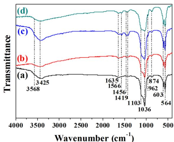
**Figure 3.** FTIR spectra of calcium phosphate nanostructures prepared by microwave-assisted hydrothermal method under different pH values: (a) Sample A, pH = 5; (b) Sample B, pH = 7; (c) Sample C, pH = 9; (d) Sample D, pH = 11.
