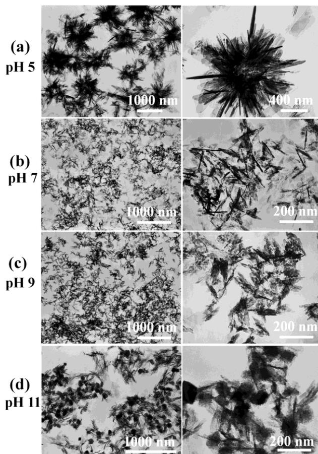
**Figure 1.** SEM of calcium phosphate nanostructures prepared with the microwave-assisted hydrothermal method under different pH values: (a) Sample A, pH = 5; (b) Sample B, pH = 7; (c) Sample C, pH = 9; (d) Sample D, pH = 11.
