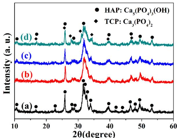
**Figure 2.** XRD patterns of calcium phosphate nanostructures prepared by microwave-assisted hydrothermal method under different pH values: (a) Sample A, pH = 5; (b) Sample B, pH = 7; (c) Sample C, pH = 9; (d) Sample D, pH = 11.
