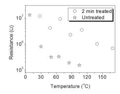
**Figure 2.** Temperature-dependent resistance of the low resistance state (LRS) memories with and without plasma treatment.
