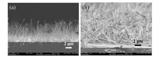
**Figure 7.** Cross-sectional scanning electron microscope (SEM) images of the ZnO NWs on the silicon substrates with gold thicknesses of (a) ~2 nm and (b) ~4 nm.
