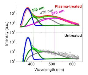
**Figure 8.** Room-temperature photoluminescence (PL) spectra of the ZnO NWs and their Gaussian components.
