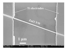
**Figure 9.** Top-view SEM images of the single ZnO NW-based resistive random access memory (RRAM) cell.
