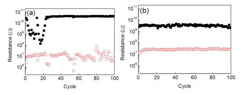
Figure 3. Endurance tests of the ZnO NW-based memories (a) without and (b) with argon plasma treatment.
