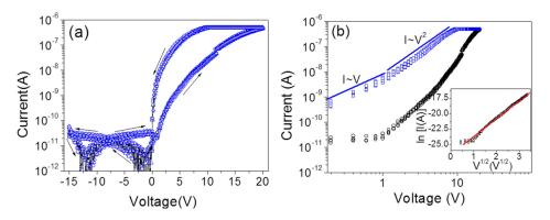
**Figure 6.** (a) Reproducible asymmetric *I*–*V* curves of single ZnO NW and (b) the *I*–*V* curves at positive bias on log-log scale with the inset fitting of  $\sqrt{V} \sim \ln(I)$  for the high resistance state (HRS).
