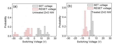
Figure 4. Distributions of switching voltages of the ZnO NW–based memories (**a**) without and (**b**) with argon plasma treatment.
