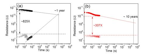
Figure 5. Data retention of the ZnO NW-based memories (a) without and (b) with argon plasma treatment.
