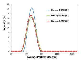
**Figure S2.** Hydrodynamic average particle sizes of the Diosarg-1,2-dioleoyl-sn-glycero-3-phosphorethanolamine (DOPE) (2:1, 1:1, 1:2) NPs in distilled water at room temperature measured by the dynamic light scattering instrument.
