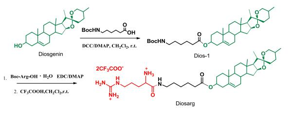
**Scheme S1.** The synthesis routes of the cationic lipid Diosarg. (DCC: N,N'-dicyclohexylcarbodiimide, EDC: 1-Ethyl-3-(3-dimethylaminopropyl)carbodiimide, DMAP: 4-Dimethylaminopyridine)
