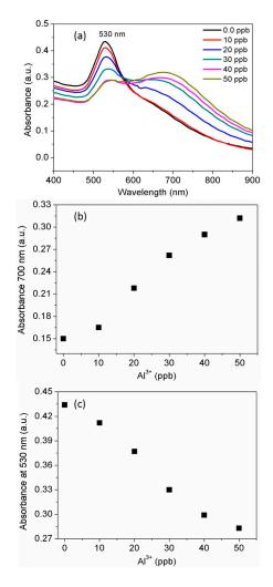
**Figure 4.** (a) The spectral response of AuNPs in the presence of increasing amounts of  $Al^{3+}$  at room temperature; (b) A linear fit curve of absorbance intensity at 700 nm vs.  $Al^{3+}$  concentration; (c) A linear fit curve of the absorbance intensity at 530 nm vs.  $Al^{3+}$  concentration.
