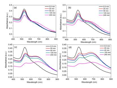
**Figure 6.** The time course of the spectral response of AuNPs at room temperature; (**a**) in the presence of the  $Al^{3+}$  (10 ppb); (**b**) in the presence of the  $Al^{3+}$  (20 ppb), (**c**) in the presence of the  $Al^{3+}$  (30 ppb); (**d**) in the presence of the  $Al^{3+}$  (40 ppb).
