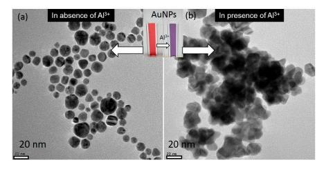
**Figure 3.** (**a**) The HR-TEM image of AuNPs in absence of  $Al^{3+}$ ; (**b**) The HR-TEM image of AuNPs in presence of  $Al^{3+}$ . (Inset showing color of corresponding AuNPs solutions).
