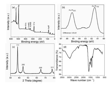
**Figure 2.** (a) XPS survey spectra of AuNPs; (b) Narrow scan spectra of AuNPs; (c) XRD spectra of AuNPs; (d) FTIR spectra of AuNPs.
