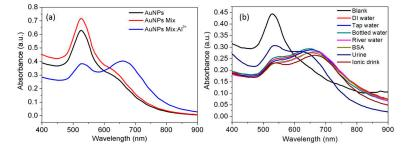
**Figure 7.** (a) The spectral response of AuNPs towards the Al<sup>3+</sup> in presence of mixture of multiple kinds of metal ions at room temperature; (b) The spectral response of AuNPs towards the Al<sup>3+</sup> in real samples at room temperature.
