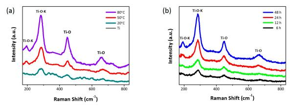
**Figure 3.** Raman spectra of Ti foils corroded (**a**) in 5 M KOH aqueous solution for 24 h at different temperatures and (**b**) in 5 M KOH aqueous solution at 50 °C for different time periods.
