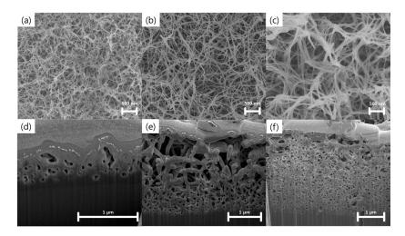
**Figure 1.** Field emission scanning electron microscopy (FE-SEM) images of the surface and cross-section of wet-corroded Ti foil at various temperatures in 5 M KOH aqueous solution: (**a**,**d**) 20 °C, (**b**,**e**) 50 °C, and (**c**,**f**) 80 °C.
