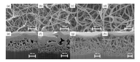
**Figure 2.** FE-SEM images of the surface and cross-section of wet-corroded Ti foil at 50 °C in 5 M KOH aqueous solution for various time periods: (**a**,**e**) 6 h, (**b**,**f**) 12 h, (**c**,**g**) 24 h, and (**d**,**h**) 48 h.
