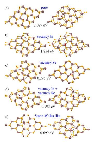
**Figure 11.** Atomic structure of pristine (a) and defective (b–e) InSe monolayer before (left) and after (right) the decomposition of the water molecules. The indicated values represent the energy cost of the dissociation of water molecules for each specific case. Reproduced with permission from Ref. [20]. Copyright Royal Society of Chemistry, 2016.
