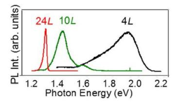
**Figure 6.** Normalized microphotoluminescence spectra for  $\gamma$ -InSe nanosheets with L=4, 10 and 24 layers. Reproduced with permission from Ref. [69].
