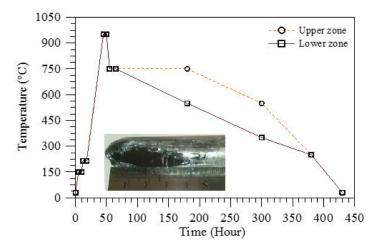
**Figure 2.** Temperature profile of the furnace in a typical Bridgman-Stockbarger growth of InSe single crystals [37]. In the inset an InSe single-crystal ingot grown by the Bridgman/Stockbarger method is displayed.
