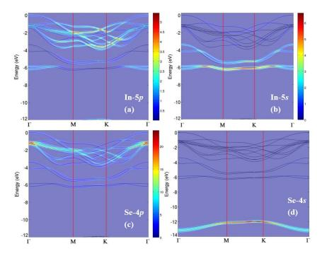
**Figure 4.** Theoretical band structure projected to (a) In-5p; (b) In-5s; (c) Se-4p; and (d) Se-4s atomic orbitals. The intensity of the various bands is reported in a color scale, whose legend is displayed in the right part of panels (a,b) and between panels (c,d). Reproduced with permission from Ref. [68].
