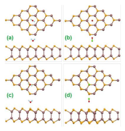
**Figure 9.** Top and side views of the geometrical structure of InSe monolayer in the case of adsorption of  $H_2O(a,c)$  and CO(b,d) molecules over hole sites (a,b) and top sites (c,d) with respect to Se atoms. Reproduced with permission from Ref. [20]. Copyright Royal Society of Chemistry, 2016.
