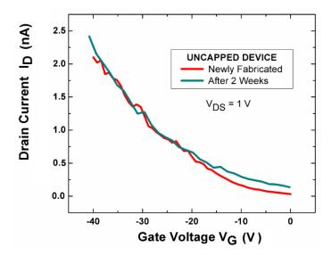
**Figure 8.**  $I_{DS}$ - $V_G$  curve of uncapped InSe-based transistors freshly fabricated (red curve) and after two weeks (blue curve). Reproduced with permission from Ref. [20]. Copyright Royal Society of Chemistry, 2016.
