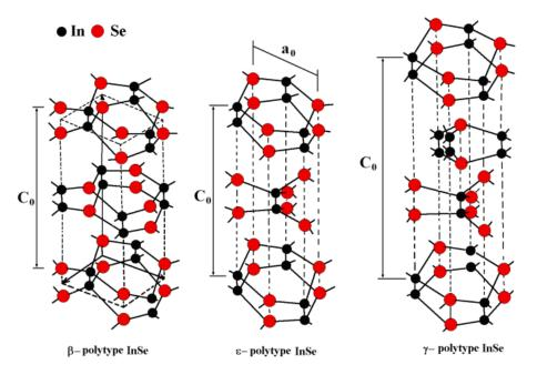
**Figure 1.** Geometrical structure of the three polytypes of InSe.  $C_0$  and  $a_0$  represent the lattice parameters along the perpendicular to layers and in the layer plane, respectively. Reproduced from Ref. [39].
