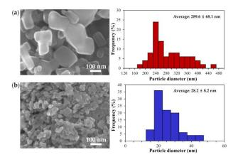
**Figure 1.** Scanning electron microscopic (SEM) images and size distribution of (**a**) bulk ZnO and (**b**) nano ZnO. Particle size distribution was determined by randomly selecting 200 particles from the SEM images.
