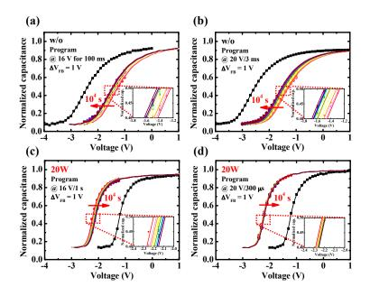
**Figure S7.** *C-V* characteristics of the w/o sample programmed at (a) 16 and (b) 20 V respectively and the 20W sample programmed at (c) 16 and (d) 20 V respectively at the retention time of  $10^4$  s. All samples were first programmed to achieve a  $\Delta V_{\rm FB}$  of 1 V. The enlarged curves of each of the samples were shown in the inset figure. The *C-V* shifts indicate the higher gate bias will improve the data retention characteristics of the 20W sample.
