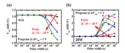
**Figure S5.** Erasing characteristics of (a) w/o and (b) 20W samples at the erasing voltages of -12 to -18 V and -14 to -26 V, respectively. All samples were first programmed to obtain a  $\Delta V_{\text{FB}}$  of 1 V. The change of  $V_{\text{FB}}$  indicates the erase of electrons and holes from Au-NPs of the w/o and 20W samples, respectively.
