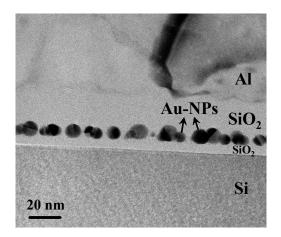
**Figure S1.** HRTEM image of the Au-NP NVMs. Distinct Au-NPs were observed on the SiO<sub>2</sub> tunneling oxide layer. The image also confirmed the film thicknesses of the TO and BO layers, for the further study of carrier injection.
