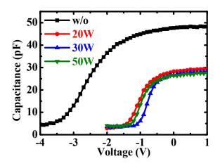
**Figure S3.** Capacitance versus voltage (C-V) characteristics of Au-NP NVMs with low-damage CF<sub>4</sub> plasma treatment on BO layer. The *C*-*V* curves were used to calculate the flat-band voltage (*V*<sub>FB</sub>) of the samples with the low-damage CF<sub>4</sub> plasma treatment on the BO layer. The *V*<sub>FB</sub> values of the samples with the low-damage CF<sub>4</sub> plasma treatment on the BO layer are roughly -1 V, which is larger than that obtained from the w/o sample.
