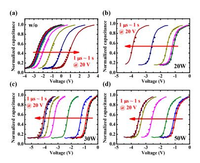
**Figure S4.** *C-V* curves of (a) w/o, (b) 20W, (c) 30W, and (d) 50W samples at the programming voltage ( $V_{g}$ - $V_{FB}$ ) of 20 V. The pulse widths were in the range of 1 µs to 1 s. The curves shift toward positive and negative directions indicate the injection of electrons from n-type Si substrate into Au-NPs and the injection of holes from Al gate into Au-NPs, respectively.
