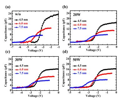
**Figure S6.** *C-V* curves of different thicknesses of SiO<sub>2</sub> films (a) without and with low-damage CF<sub>4</sub> plasma treatment of (b) 20 W, (c) 30 W, and (d) 50 W. The SiO<sub>2</sub> films with the thicknesses of 4.5, 6.0, and 7.5 nm were deposited by the PECVD system. These curves were used to extract the effective work-function of Al gate on the CF<sub>4</sub>-plasma-treated SiO<sub>2</sub> films.
