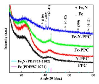
Figure 1. X-ray diffraction (XRD) patterns of PPC, N-PPC, Fe-PPC, and Fe-N-PPC carbonized at 900 °C.
