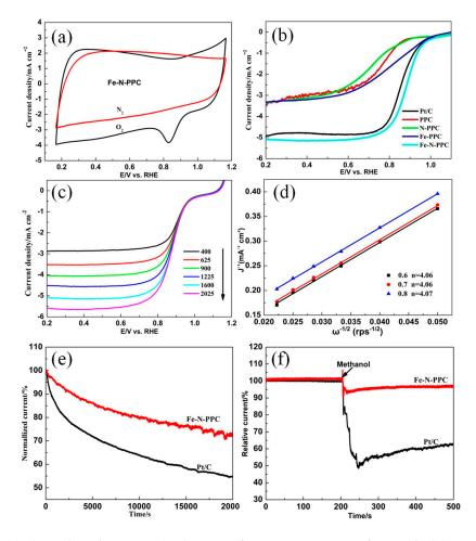
**Figure 5.** (a) The cyclic voltammetry (CV) curves of Fe-N-PPC at a scan of 50 mV/s; (b) LSV curves of PPC and other samples at a scan rate of 10 mV/s and an electrode rotation rate of 1600 rpm; (c) LSV curves of Fe-N-PPC at various rotation rates and a scan rate of 10 mV/s; (d) Corresponding K–L plots at different potentials; (e) Long-term stability test of Fe-N-PPC and 20% Pt/C in a 0.1 M KOH solution; (f) Methanol (3 M) crossover resistance test.
