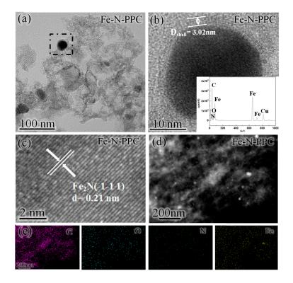
**Figure 4.** (a) Transmission electron microscopy (TEM) images; (b,c) energy dispersive X-ray spectroscopy (EDS) patterns and high resolution TEM (HRTEM) images of Fe-N-PPC; (d) high-angle annular dark-field scanning transmission electron microscopy (HAADF-STEM) image and (e) EDS elemental mapping images (C, O, N and Fe) of Fe-N-PPC.
