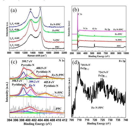
**Figure 2.** (a) Raman spectra and (b) High-resolution X-ray photoelectron spectroscopy (XPS) spectra of PPC, N-PPC, Fe-PPC, and Fe-N-PPC; (c) N 1s spectra of PPC, N-PPC and Fe-N-PPC; (d) Fe 2p spectra of Fe-N-PPC.
