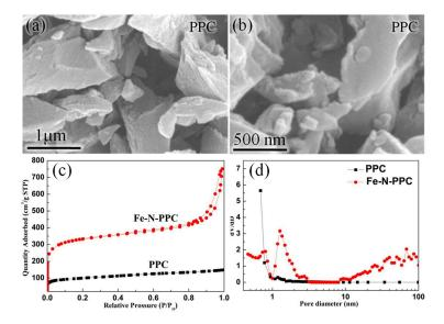
Figure 3. (a,b) Scanning electron microscopy (SEM) images of PPC; (c)  $N_2$  adsorption–desorption isotherms and (d) Pore size distributions of PPC and Fe-N-PPC respectively.
