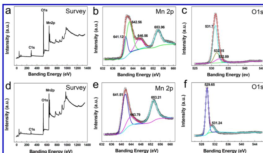
**Figure S3.** XPS spectra of  $\text{MnCO}_3$  precursor and  $\text{GC@Mn}_2\text{O}_3$  microspheres Surveys of (a)  $\text{MnCO}_3$  and (d)  $\text{GC@Mn}_2\text{O}_3$  microspheres, Mn-2p core-level XPS spectra of (b)  $\text{MnCO}_3$  and (e)  $\text{GC@Mn}_2\text{O}_3$ , and O-1s core-level XPS spectra of (c)  $\text{MnCO}_3$  and (f)  $\text{GC@Mn}_2\text{O}_3$ .
