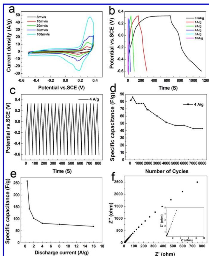
**Figure S5.** Electrochemical properties of electrodes made with monodispersed microspheres after annealed at 400 °C. (a) CV curves at different scan rates, (b) galvanostatic charge/discharge curves at
