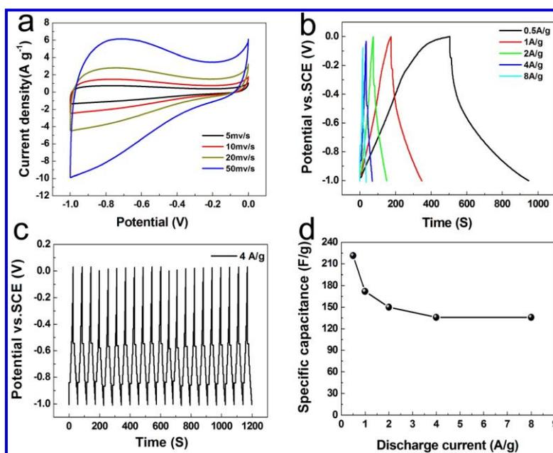
**Figure S4.** Electrochemical properties of electrodes made with active carbon. (a) CV curves at different scan rates, (b) galvanostatic charge/discharge curves at different current densities, (c) cycle stability at current density of 4 A g<sup>-1</sup>, and specific capacitances at different current densities.
