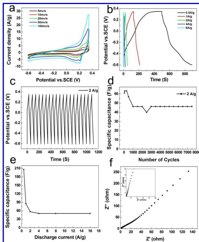
**Figure S6.** The electrochemical properties of electrodes made with monodispersed microspheres after annealed at 600 °C. (a) CV curves at different scan rates, (b) galvanostatic charge/discharge curves at different current densities, (c,d) cycle stability at current density of 2 A g<sup>-1</sup>, (e) specific capacitances at different current densities and (f) EIS spectrum.
