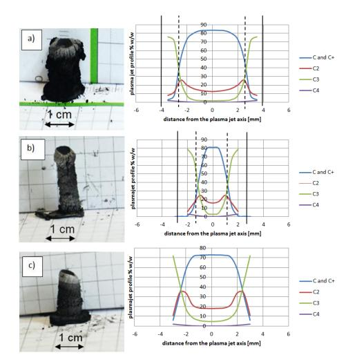
**Figure 14.** Examples of cathode deposits (photos in the left and plasma column composition in the right) where (**a**) Ni as catalyst (5 wt %, pressure 200 hPa, current 90 A, voltage 26 V); (**b**) Y as catalyst (5 wt %, pressure 200 hPa, current 60 A, voltage 25 V); (**c**) Fe as catalyst (5 wt %, pressure 200 hPa, current 70 A, voltage 22.5 V).
