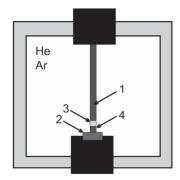
**Figure 1.** Arc discharge carbon nanotubes synthesis system where: 1—anode; 2—cathode; 3—vapour jet; 4—cathode deposit.
