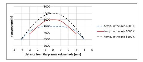
**Figure 11.** Examples of temperature profiles with average temperature in the axis: 4500 K, 5000 K and 5500 K (for the distance between electrodes -2 mm; pressure 200 hPa; helium as an inert gas; current 70 A, 80 A, 90 A respectively).
