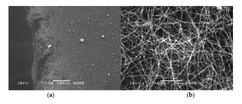
**Figure 5.** Scanning electron microscopy (SEM) analysis of the sample with carbon nanotubes after oxidation (pressure 200 hPa, current 80 A, voltage 21 V). Figures shows different magnification of the sample— $100 \times$  on (**a**);  $5000 \times$  on (**b**).
