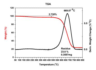
**Figure 3.** Thermogravimetric analysis (TGA) of the sample with carbon nanotubes with iron nanoparticles after oxidation (example for 5% w/w iron as catalyst, pressure 200 hPa, current 70 A, voltage 22.5 V).
