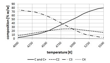
Figure 10. Decomposition of carbon at temperatures 4000–5500 K.
