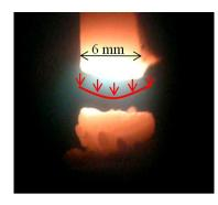
Figure 7. Plasma column gap in arc plasma carbon nanotubes (CNTs) synthesis.
