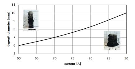
Figure 13. Influence of the discharge current on deposit size.
