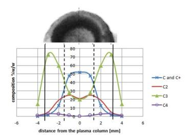
Figure 12. Plasma column composition with carbon deposit structure (top). Deposit obtained under conditions: pressure 300 hPa, current 80 A, voltage 20.5 V.
