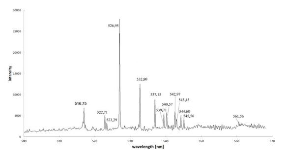
**Figure 8.** Spectra for arc discharge in the discharge axis during carbon nanotubes synthesis supported by iron as a catalyst (recorded by Stellarnet HR-NIR4, Stellarnet Inc., Tampa, FL, USA, spectrometer).
