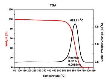
**Figure 4.** TGA analysis of the sample with carbon nanotubes after oxidation (pressure 200 hPa, current 80 A, voltage 21 V).
