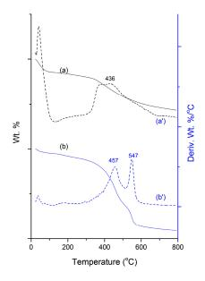
**Figure 2.** Thermogravimetric analysis (TGA) spectra of (**a**) MSN-NH<sub>2</sub>; and (**b**) MSN-HCD and their respective derivative weight loss curves (**a**',**b**'). Mesoporous silica nanoparticles (MSN)-NH<sub>2</sub>; 16-hydroxycleroda-3,13-dine-16,15-olide (HCD).
