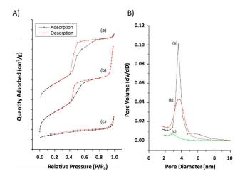
**Figure 3.** Nitrogen adsorption–desorption isotherms (**A**) and their respective distribution curves of Barret-Joyner-Halenda (BJH) pore size (**B**) of MSNs and conjugated-MSNs. (**a**) MSN; (**b**) MSN-NH<sub>2</sub>; and (**c**) MSN-HCD. Mesoporous silica nanoparticles (MSN)-NH<sub>2</sub>; 16-hydroxycleroda-3, 13-dine-16,15-olide (HCD).
