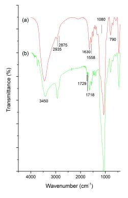
**Figure 1.** Fourier transform infra-red (FT-IR) spectra of (**a**) mesoporous silica nanoparticles (MSN)-NH<sub>2</sub>; and (**b**) MSN-HCD. (16-hydroxycleroda-3,13-dine-16,15-olide, HCD).
