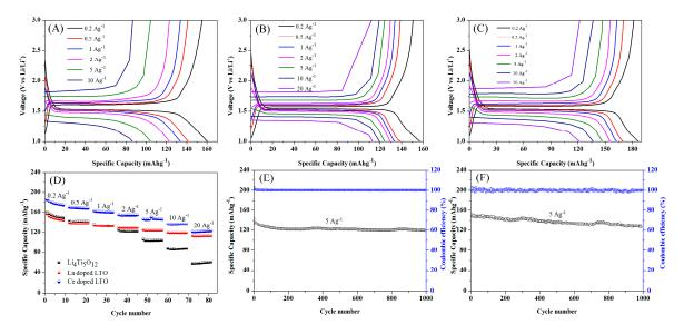
**Figure 5.** The galvanostatic discharge-charge profiles of pure LTO (**A**), La-doped LTO (**B**) and Ce-doped LTO (**C**) at varied current density; (**D**) Rate performance for these samples (**E**); Cycle performance plots of La-doped LTO (**E**) and Ce-doped LTO (**F**) at  $5 \text{ Ag}^{-1}$ .
