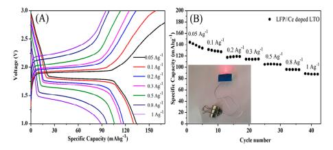
**Figure 9.** (**A**) Galvanostatic charge-discharge voltage profiles of a LiFePO<sub>4</sub>/Ce-doped LTO full cell at varied current densities within a voltage of 1–3 V; (**B**) The rate performance for LiFePO<sub>4</sub>/Ce doped LTO full cell (inset: digital picture of a light-emitting diode (LED) powered by an as-fabricated full cell).
