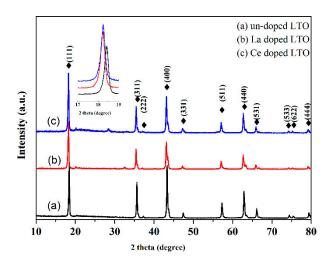
**Figure 1.** X-ray diffraction (XRD) patterns of pure  $\text{Li}_4\text{Ti}_5\text{O}_{12}$  (LTO), undoped LTO (**a**), La-doped LTO (**b**) and Ce-doped LTO (**c**).
