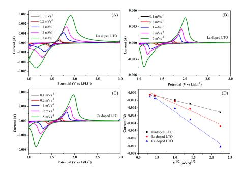
**Figure 6.** Cyclic voltammetry (CV) curves of undoped LTO (**A**); La-doped LTO (**B**); Ce-doped LTO (**C**); at varied scanning rates from 0.1 to 5.0 mV/s; The cathodic peak currents against square roots of scan rate (**D**).
