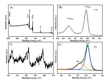
**Figure 4.** X-ray photoelectron spectroscopy (XPS) survey of Ce-doped LTO (**A**), Ti 2p (**B**), Ce 3d (**C**) and O 1s (**D**).
