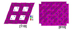
**Figure 7.** LTO crystal structure view from  $[\bar{1}10]$  and [010].
