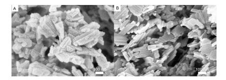
Figure 2. Scanning electron microscopy (SEM) images of undoped LTO (A) and Ce-doped LTO (B).
