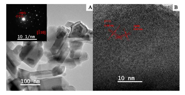
**Figure 3.** TEM image (**A**) and high resolution (HR)TEM image (**B**) of Ce-doped LTO [inset of A, the corresponding selected area electronic diffraction (SAED) pattern].
