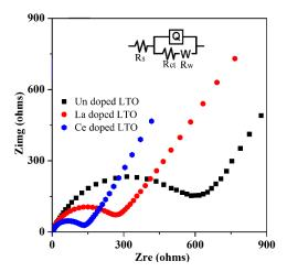
**Figure 8.** Electrochemical impedance spectra of Ce/La-doped LTO, undoped LTO and pure  $\text{Li}_4\text{Ti}_5\text{O}_{12}$  electrodes (inset shows the equivalent circuit).
