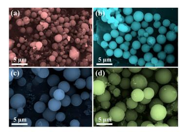
Figure 1. SEM images of CPCMs prepared at (a) 140 °C; (b) 160 °C; (c) 180 °C; and (d) 200 °C.
