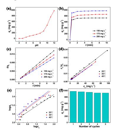
**Figure 3.** Effect of (**a**) pH ( $c_0$ : 200 mg L<sup>-1</sup>, 2 h, 25 °C), (**b**) contact time ( $c_0$ : 150, 175 and 200 mg L<sup>-1</sup>, pH: 12, 25 °C), (**c**) pseudo-second-order kinetics, and (**d**–**e**) Langmuir and Freundlich isotherms of MB adsorption on CPCMs; (**f**) The reusability of CPCMs toward MB adsorption ( $c_0$ : 200 mg L<sup>-1</sup>, pH: 12).
