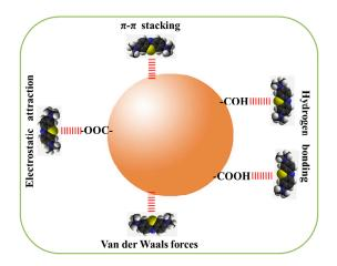
Figure 4. A potential mechanism for MB adsorption on CPCMs.
