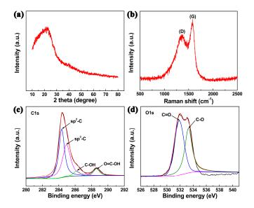
**Figure 2.** (**a**) XRD pattern, (**b**) Raman spectrum, and (**c**,**d**) high-resolution XPS spectra of C1s and O1s of CPCMs.
