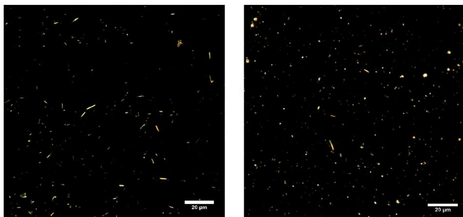
**Figure 5.** DF optical images of HNTs (left) and HNTs/ $\text{Ca}(\text{OH})_2$  (right) with calcium phosphate end-stoppers in water.
