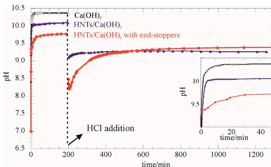
**Figure 7.** pH measurements in aqueous dispersion before and after HCl solution addition as functions of time. The inset reports an enlargement of the initial release.
