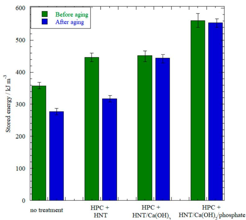
**Figure 8.** Stored energy up to sample breaking from tensile stress measurements. The error is based on the standard deviation from repeated experiments.
