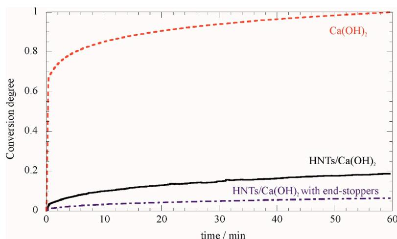
**Figure 6.** Degree of  $\text{Ca}(\text{OH})_2$  carbonation in a  $\text{CO}_2$  atmosphere for  $\text{Ca}(\text{OH})_2$ , HNT/ $\text{Ca}(\text{OH})_2$  and HNT/ $\text{Ca}(\text{OH})_2$  with phosphate end-stoppers.
