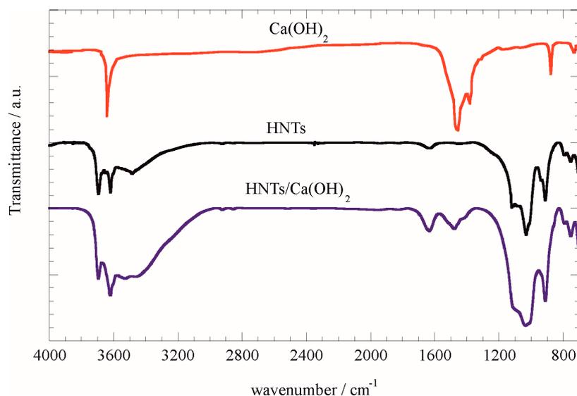
Figure 1. FTIR spectra for  $\text{Ca}(\text{OH})_2$ , HNTs and HNTs/ $\text{Ca}(\text{OH})_2$ .
