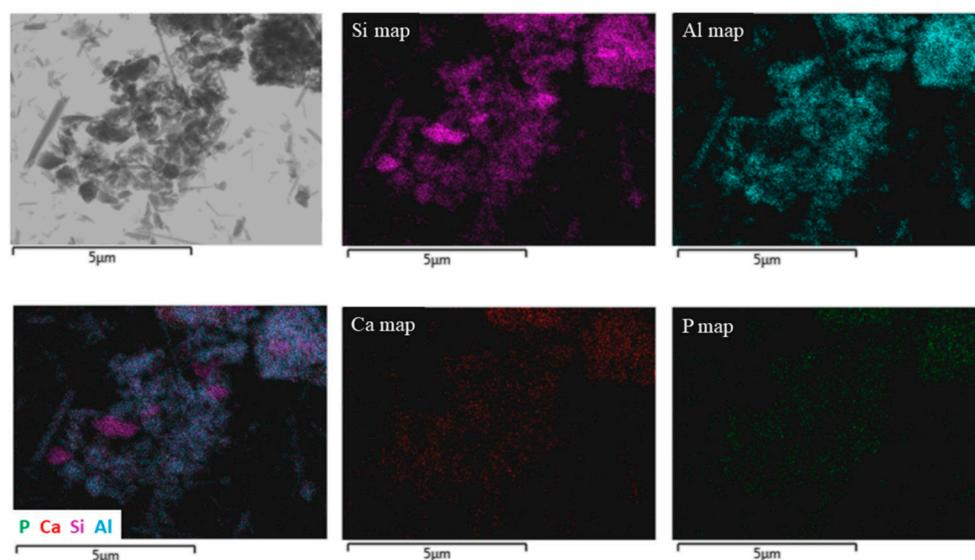
Figure 3. TEM image and EDX mapping of HNTs/ $\text{Ca}(\text{OH})_2$  with calcium phosphate end-stoppers.
