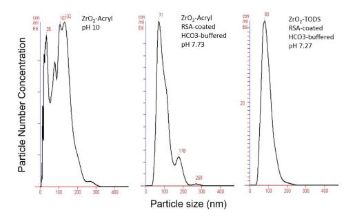
**Figure S2.** Size distribution of rat serum albumin-coated ZrO<sub>2</sub> particles as prepared for intratracheal administration in rats. Particles were buffered with 25 mM HCO<sub>3</sub><sup>-</sup> and 5% CO<sub>2</sub>. Measurements were carried out with optical particle tracking and NanoSight Software NTA 2.2 (Minton Park Amesbury, Wiltshire SP4 7RT, UK).
