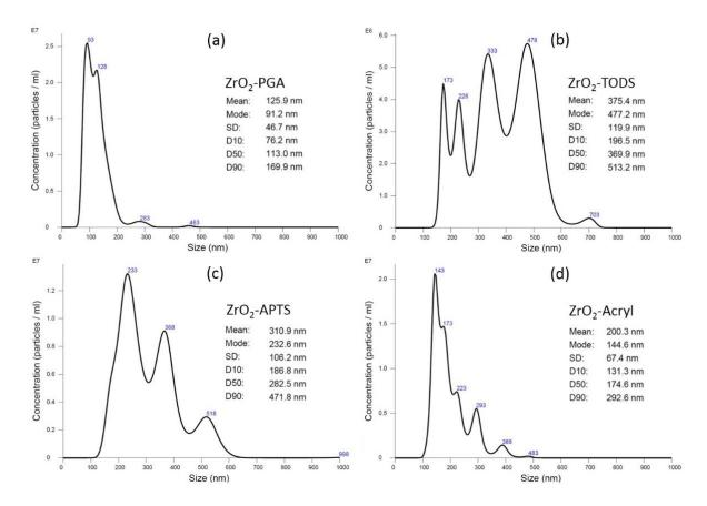
**Figure S3.** Size distribution of ZrO<sub>2</sub> nanoparticles dispersed in 0.9% NaCl/PBS as used for an administration study in ovalbumin-sensitized mice. (a) ZrO<sub>2</sub>-PGA, (b) ZrO<sub>2</sub>-TODS, (c) ZrO<sub>2</sub>-APTS, and (d) ZrO<sub>2</sub>-Acryl. Measurements were carried out with optical particle tracking and NanoSight Software NTA 3.1 (Minton Park Amesbury, Wiltshire SP4 7RT, UK).
