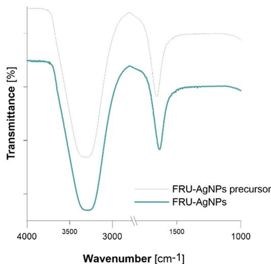
**Figure 6.** ATR FT-IR spectra of the working solution before (FRU-AgNPs precursor) and after (FRU-AgNPs) dc-APGD treatment.
