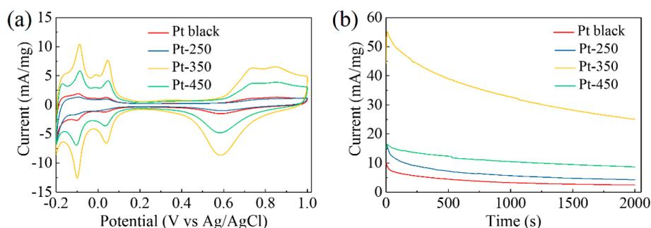
**Figure 4.** (a) Cyclic voltammograms were carried out in 0.5 M H<sub>2</sub>SO<sub>4</sub> with the potential between -0.2 and 1 V at a scan rate of 50 mV·s<sup>-1</sup>. (b) Chronoamperometric curves at 0.6 V were recorded in an aqueous solution containing 0.5 M H<sub>2</sub>SO<sub>4</sub> and 0.5 M CH<sub>3</sub>OH.
