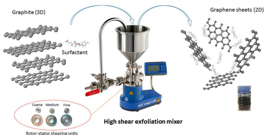
**Figure 30.** Schematic illustration of the exfoliation process using a high shear colloidal mixer. Reproduced from [24]. Copyright Springer, 2017.
