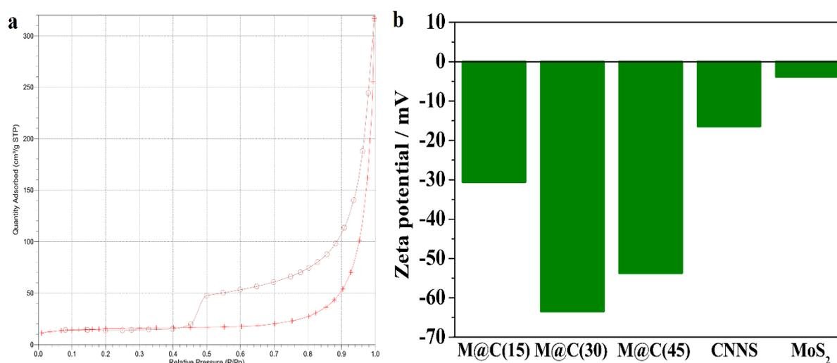
**Figure S1.** Adsorption/desorption isotherms of MoS<sub>2</sub>@CNNS(30) (a) and zeta potentials of the MoS<sub>2</sub>@CNNS nanocomposites dispersed in ultrapure water (pH = 4.0) (b).
