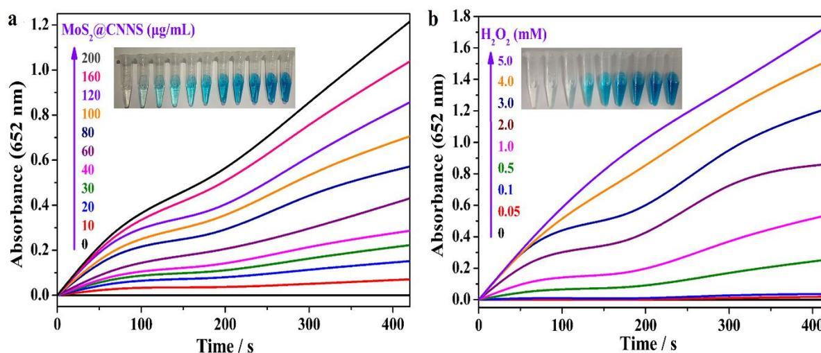
**Figure S2.** Time-dependent absorbance at 652 nm and color changes of 0.8 mM TMB reaction solutions in the absence or presence of different concentrations of MoS<sub>2</sub>@CNNS(30) (a) and H<sub>2</sub>O<sub>2</sub> (b) in 25.0 mM PBS (pH = 4.0) at room temperature. Inset: related color variations.
