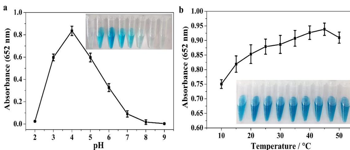
**Figure S3.** Dependency of peroxidase-like activity of MoS<sub>2</sub>@CNNS(30) on pH (a) and temperature (b) and color changes. Experiments were conducted by using 120 µg/mL of MoS<sub>2</sub>@CNNS(30) in 25.0 mM PBS with 2.0 mM H<sub>2</sub>O<sub>2</sub> and 0.8 mM TMB as substrates. Inset: related color variations.
