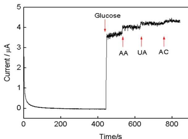
**Figure 8.** Typical current-time curve recorded at a PPy-RGO-(AuNPs-GOD)<sub>4</sub>/GCE during the addition of glucose, ascorbic acid (AA), uric acid (UA), and acetaminophen (AC) at a potential of 0.5 V versus SCE.
