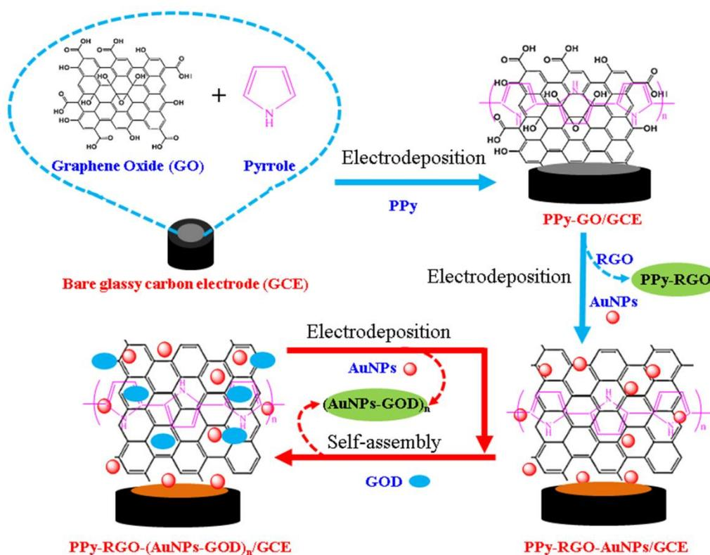
**Figure 1.** Schematic illustration of a glucose biosensor using the polypyrrole and reduced graphene oxide (PPy-RGO), and gold nanoparticles and glucose oxidase (AuNPs-GOD) multilayer films as the sensitive layer fabricated by the electrodeposition and self-assembly.
