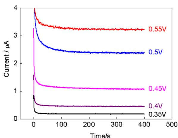
**Figure 6.** Current-time curves for PPy-RGO-(AuNPs-GOD)<sub>4</sub>/GCE in 4 mM glucose at different applied potentials from 0.35 V to 0.55 V versus SCE.
