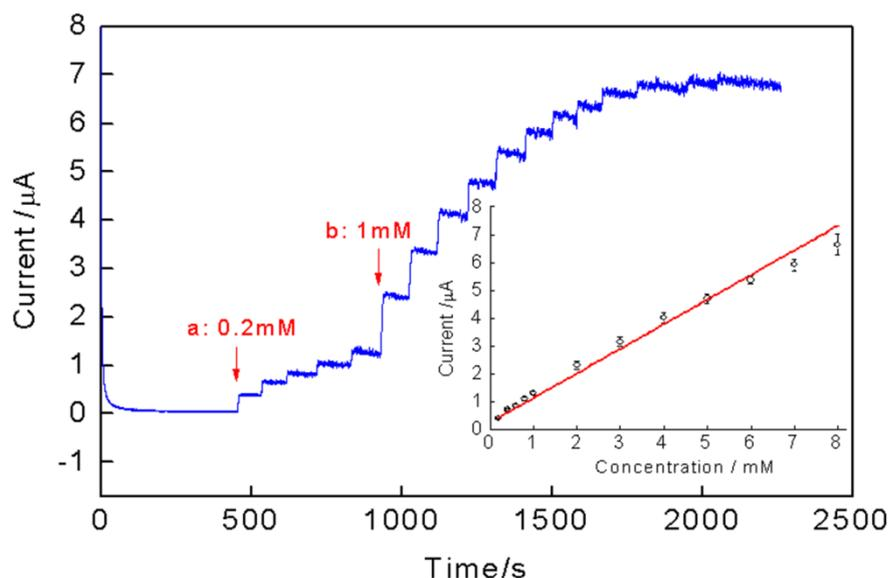
**Figure 7.** Typical current-time curve recorded at a PPy-RGO-(AuNPs-GOD)<sub>4</sub>/GCE during the addition of different concentration glucose (0.2 mM–13 mM) at a potential of 0.5 V versus SCE. The arrows “a” and “b” indicated each increased glucose concentration is 0.2 mM and 1 mM, respectively. Inset: the calibration curve of the electrode with glucose concentration ranged from 0.2 mM to 8 mM. Error bar = standard deviation ( $n = 5$ ).
