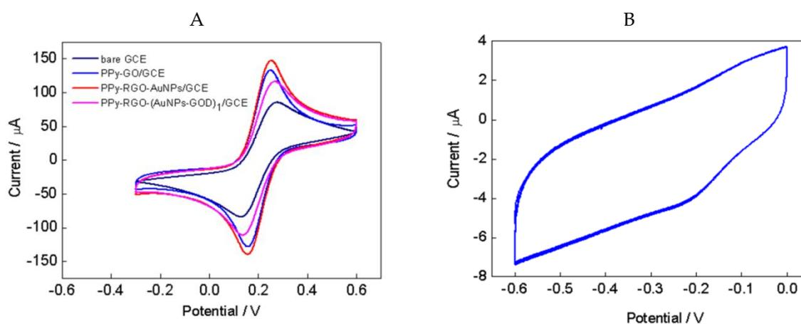
**Figure 4.** (A) CVs of the electrode at different stages: bare GCE; PPy-GO/GCE; PPy-RGO-AuNPs/GCE; and PPy-RGO-(AuNPs-GOD)<sub>1</sub>/GCE. Supporting electrolyte, 0.1 M KCl containing 5mM [Fe (CN)<sub>6</sub>]<sup>3−/4−</sup> (1:1). (B) CVs of PPy-RGO-(AuNPs-GOD)<sub>1</sub>/GCE recorded in pH 7.0 phosphate buffer solutions. Scan rate, 50 mV/s.
