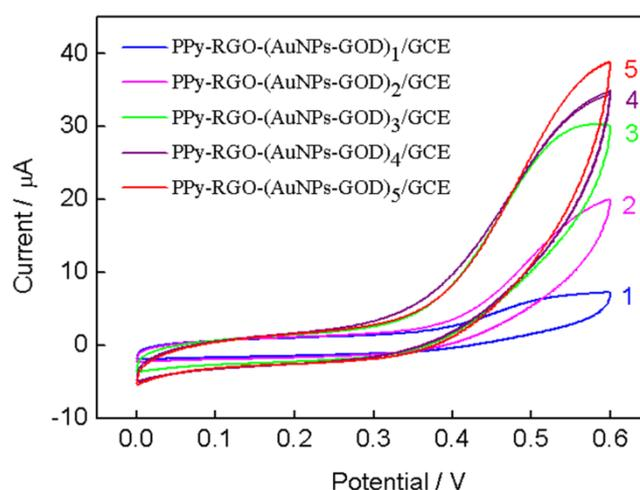
**Figure 5.** CVs of different layers of AuNPs-GOD multilayer films modified PPy-RGO/GCE in 10 mM glucose. The layer number of multilayer films was indicated on the graph. Scan rate, 50 mV/S.
