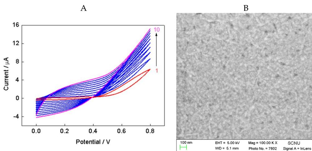
**Figure 2.** Cyclic voltammograms (CVs) of bare glassy carbon electrode (GCE) in pyrrole/graphene oxide solution for 10 cycles with a scan rate of 25 mV/s (A) and typical SEM image of polypyrrole (PPy)/graphene oxide (GO) (B).
