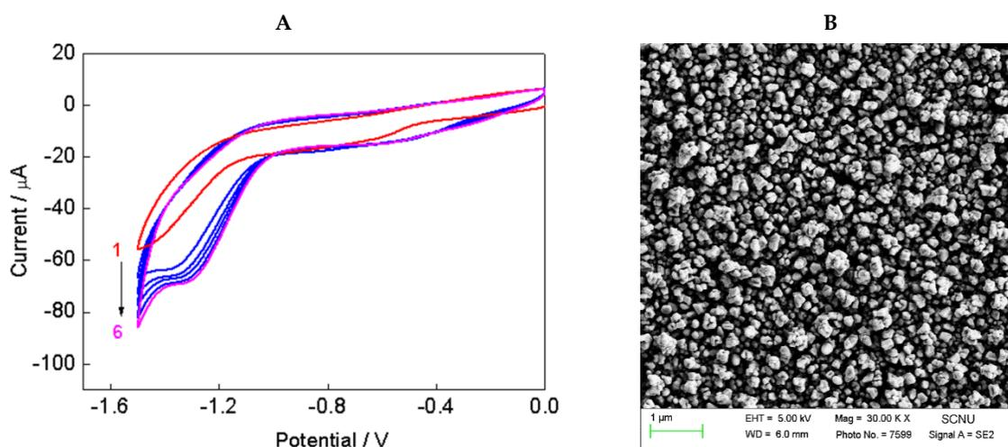
**Figure 3.** CVs of PPy-GO/GCE electrode in  $\text{HAuCl}_4$  aqueous solution for 6 cycles with a scan rate of 25 mV/s (A), and the typical SEM image of PPy-RGO-AuNPs (B).
