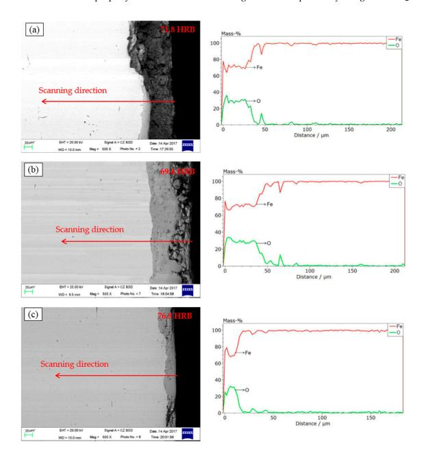
**Figure 7.** SEM images and EDS spectra of oxide scales of hot-rolled strips lubricated with (a) non-lubricant; (b) traditional lubricating fluid and (c) nano-TiO<sub>2</sub> fluid.
