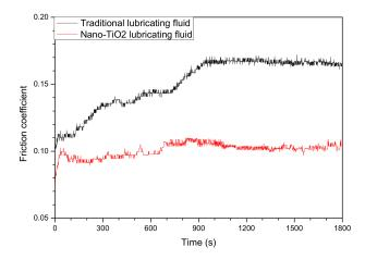
Figure 3. Friction coefficient-time curves of traditional lubricating fluid and nano-TiO<sub>2</sub> fluid.
