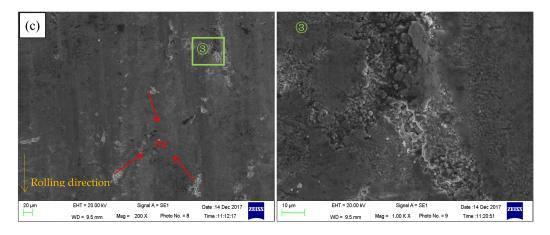
**Figure 5.** SEM images of hot-rolled surfaces lubricated with (**a**) non-lubricant; (**b**) traditional lubricating fluid and (**c**) nano-TiO<sub>2</sub> fluid.
