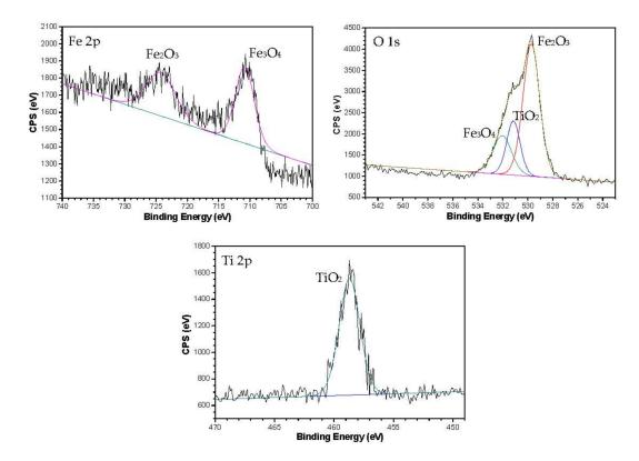
Figure 8. XPS spectra of Fe 2p, O 1s and Ti 2p on the oxide scales surface lubricated with nano-TiO<sub>2</sub> fluid.
