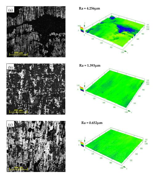
**Figure 4.** Optical micrograph and 3D topography of hot-rolled surface lubricated with (**a**) non-lubricant; (**b**) traditional lubricating fluid and (**c**) nano-TiO<sub>2</sub>lubricating fluid.
