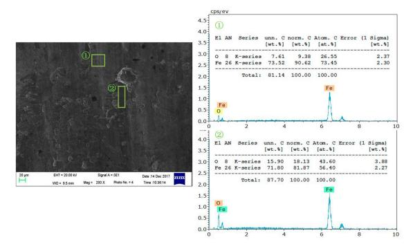
**Figure 6.** Energy dispersive spectrometry (EDS) spectra of strip surface lubricated with traditional lubricating fluid.
