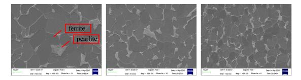
**Figure 9.** Microstructures of rolled strips for (**a**) non-lubricant; (**b**) traditional lubricating fluid and (**c**) nano-TiO<sub>2</sub>lubricating fluid.
