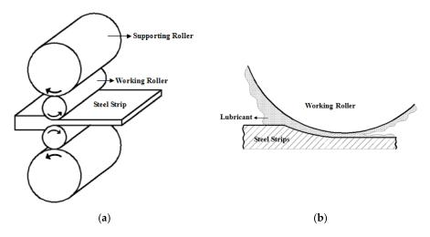
Figure 2. Sketches of (a) hot rolling and (b) lubrication during hot rolling.
