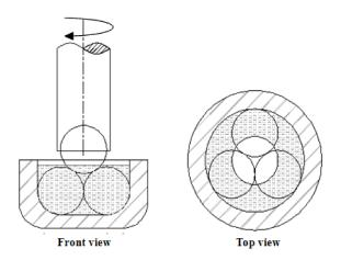
Figure 1. Schematic of the four-ball rolling friction.
