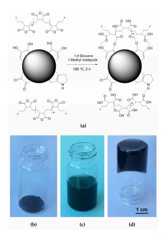
**Figure 1.** (**a**) Schematic representation of the synthetic approach and proposed structure for our sepia melanin-P(E-*alt*-MA) hybrid. Melanin is represented as a black pearl with protruding functional groups and dashed lines represent hydrogen bonds; (**b**) Photograph of the as-prepared hybrid; (**c**,**d**) Photographs of the gel obtained upon addition of water to powdered hybrid.
