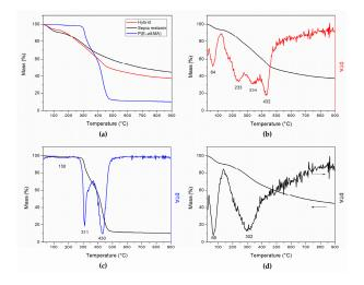
**Figure 3.** (a) Summary of the thermogravimetric plots; (b) TGA and DTA analysis of the sepia melanin-P(E-*alt*-MA) hybrid; (c) TGA and DTA analysis of P(E-*alt*-MA); (d) TGA and DTA analysis of sepia melanin.
