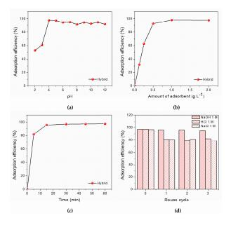
**Figure 4.** Evaluation of the adsorption efficiency of the sepia melanin-P(E-*alt*-MA) hybrid (**a**) as a function of pH; (**b**) as a function of the adsorbent's amount; (**c**) as a function of time; (**d**) as a function of reuse cycle with different desorbing agents. All data shown are the average of three independent measurements, the relative standard deviation being  $\leq 10\%$ . The lines are a guide for the eye.
