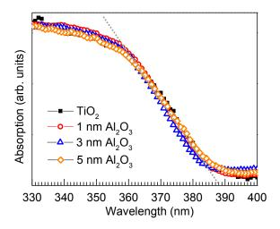
**Figure 4.** Absorption spectra of pristine anatase TiO<sub>2</sub> powder and the TiO<sub>2</sub> coated with Al<sub>2</sub>O<sub>3</sub> films with different thicknesses: 1 nm, 3 nm, and 5 nm.
