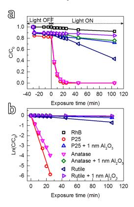
**Figure 7.** (a) Photodegradation as a function of exposure time of RhB solution by uncoated  $TiO_2$  (P25, anatase and rutile) and the  $TiO_2$  coated with 1 nm  $Al_2O_3$ , and (b) the corresponding kinetic plots. All of the photocatalytic tests were carried out under identical experimental conditions. The self-degradation of RhB is added as the reference.
