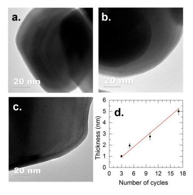
**Figure 1.** TEM images of  $Al_2O_3$  films deposited on anatase  $TiO_2$  nanoparticles for (a) three cycles, (b) 10 cycles and (c) 17 cycles, and (d) the coating thickness as a function of the number of cycles.
