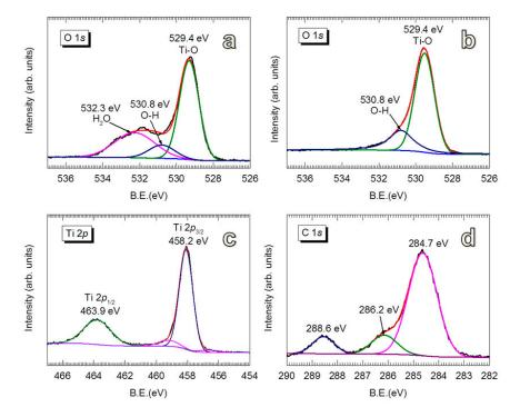
**Figure 2.** XPS spectra of uncoated anatase  $TiO_2$  powders: O 1s (a) without and (b) with preheating (at 170 °C in air), (c) Ti 2p and (d) C 1s.
