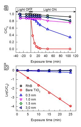
**Figure 6.** (a) Photodegradation of RhB solution using anatase TiO<sub>2</sub> coated with Al<sub>2</sub>O<sub>3</sub> films with different thicknesses as a function of exposure time, and (b) the corresponding kinetic reaction plots.
