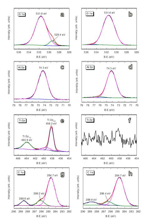
**Figure 3.** XPS spectra of anatase  $TiO_2$  coated with 3 nm thick (**a**,**c**,**e**,**g**—on the left side) and 5 nm thick (**b**,**d**,**f**,**h**—on the right side)  $Al_2O_3$  films.
