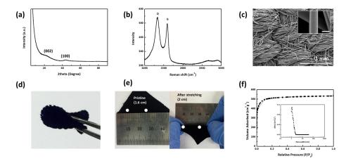
**Figure 1.** Structural characterization of the carbon cloth (CC). (a) XRD pattern; (b) Raman spectrum; (c) SEM images (scale bar of inset image:  $10 \ \mu$ m); photo images of (d) folded and (e) stretched CC support; (f) N<sub>2</sub> sorption isotherm; and (f, inset) the corresponding pore size distribution calculated by the NLDFT method.
