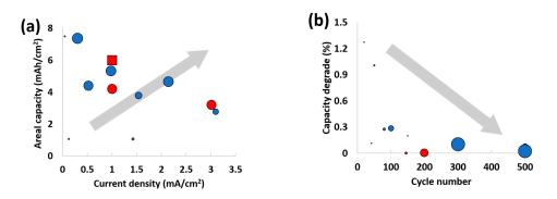
**Figure 5.** Ragone plots of (**a**) areal current density vs. areal capacity (mean of diameter: amount of sulfur loading) and (**b**) cycle number vs. capacity degrade (mean of diameter: C rate). Circle and square dots mean coin cell and pouch cell data, respectively. Dots in red represent data from this work.
