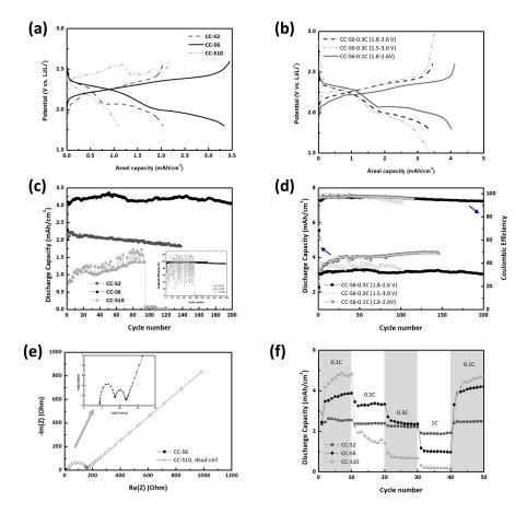
**Figure 3.** Charge/discharge profiles at the 50th cycle and cycle stability. (**a**,**c**) CC-S2, CC-S6, and CC–S10 operated at C/3 and (**b**,**d**) CC-S6 at C/3 and C/10 in the potential range of 1.8–2.6 and 1.5–3.0 V vs. Li/Li<sup>+</sup>; (**e**) EIS spectra of CC-S6 and CC-S10 after GCPL cycling at C/3; (**f**) Rate capability of CC-S between C/10 and 1 C.
