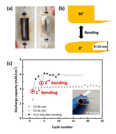
**Figure 4.** (a) Photo images of 2 cm  $\times$  6 cm pouch cell showing the CC electrode (left) and the Li metal anode (right); (b) Scheme of the pouch cell bending test condition; (c) Cycle stability of the pouch and coin cells in the potential range of 1.5–3.0 V vs. Li/Li<sup>+</sup> at C/10 (inset photo image shows the pouch cell bended at 0°).
