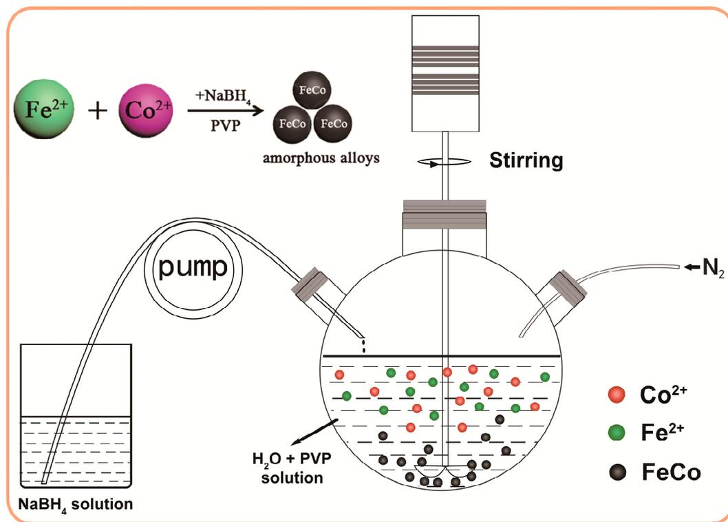
**Figure 1.** The schematic formation process for the amorphous FeCo nanoalloys.
