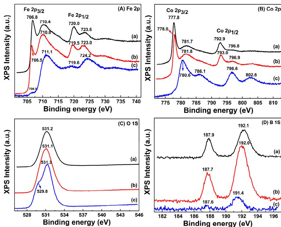
**Figure 6.** The XPS narrow-scan spectra of Fe 2p (A), Co 2p (B), O 1s (C) and B 1s (D) for amorphous FeCo nanoalloys prepared with different PVP additions of 1.5 g (a), 2 g (b) and the sample prepared without PVP (c).
