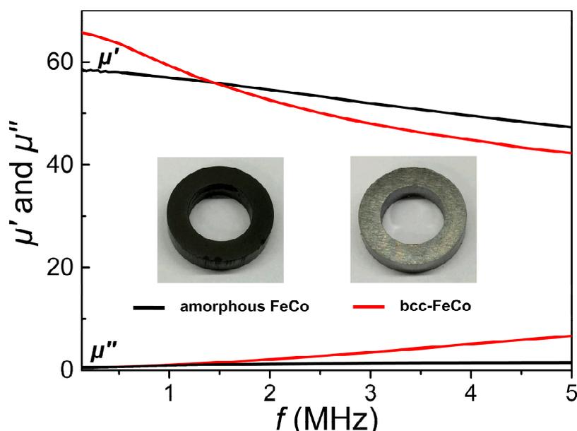
**Figure 8.** The complex permeability spectra for the two compacted samples of the amorphous FeCo prepared with 1.5 g PVP additions and high-purity Fe<sub>65</sub>Co<sub>35</sub> particles.
