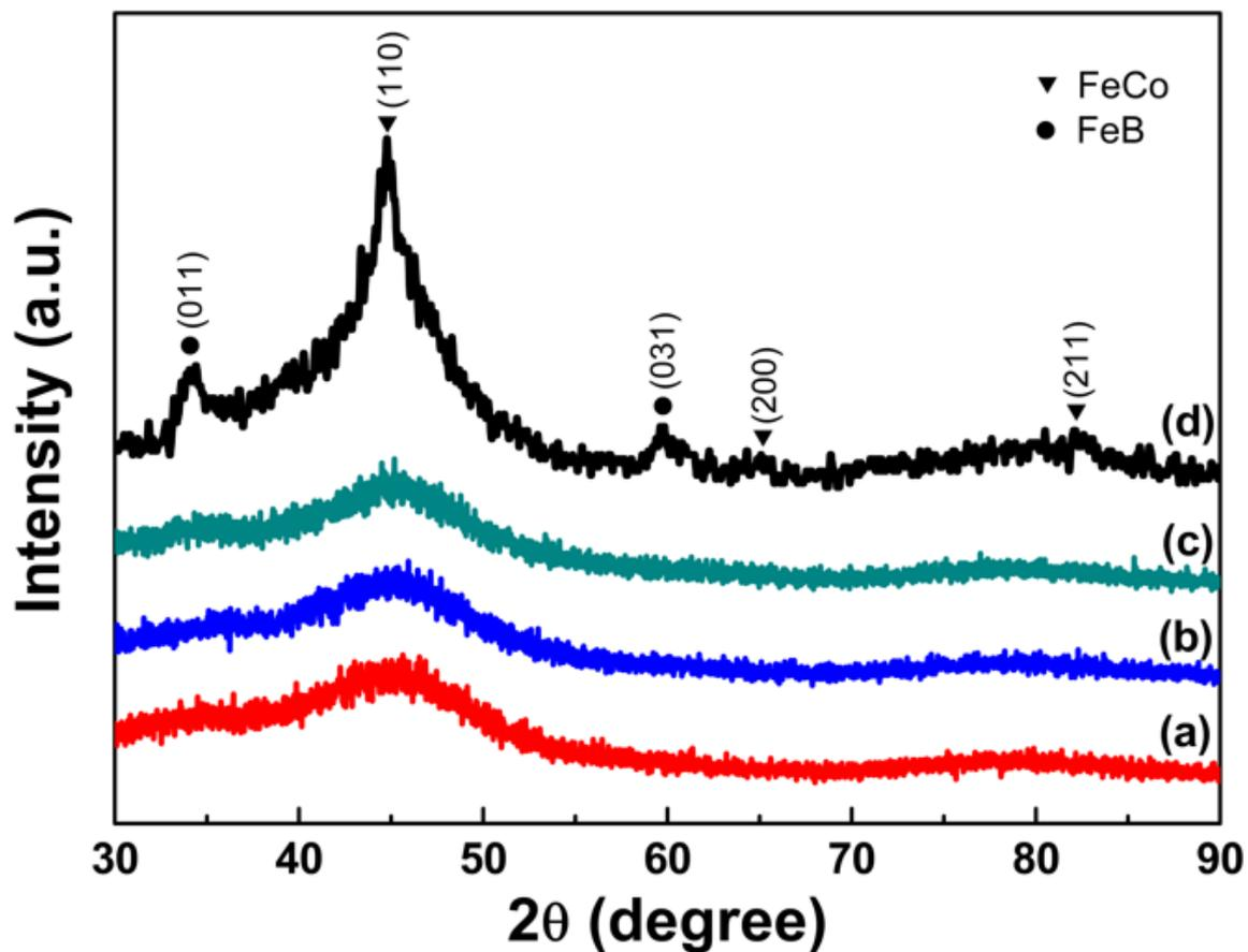
**Figure 2.** The X-ray diffraction (XRD) patterns of as-synthesized samples prepared with different PVP additions of 1 g (a), 1.5 g (b), 2 g (c) and without PVP (d).
