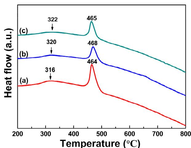
**Figure 4.** The DSC measurement of amorphous FeCo nanoparticles prepared with different PVP additions of 1 g (a), 1.5 g (b) and 2 g (c).
