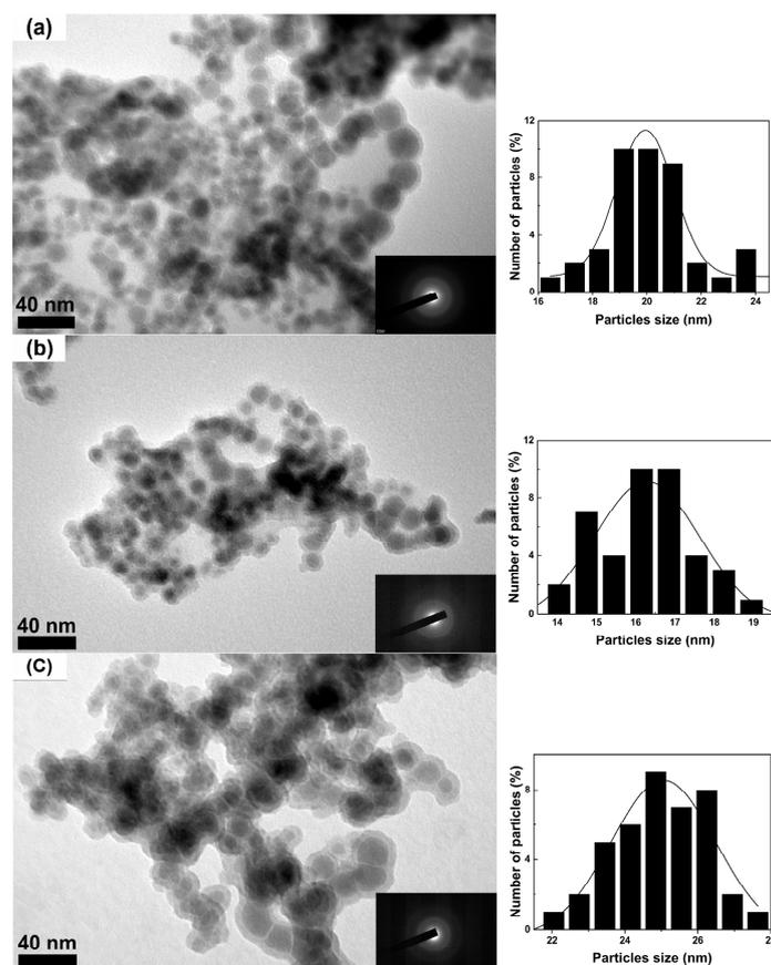
**Figure 3.** The representative transmission electron microscope (TEM) micrographs and the selected-area electron diffraction (SAED) patterns along with the corresponding histograms on the right side of the figure for amorphous FeCo nanoparticles prepared with different PVP additions of 1 g (a); 1.5 g (b) and 2 g (c).
