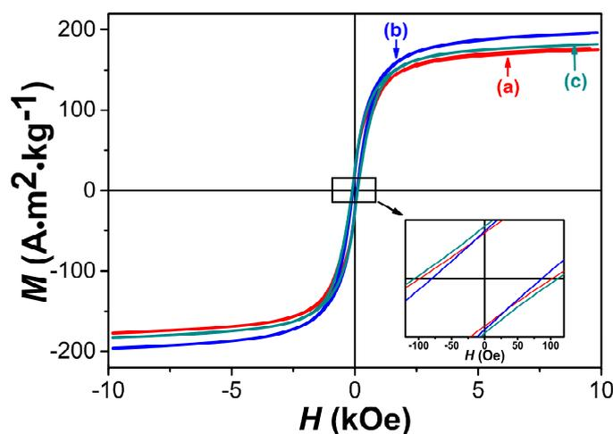
**Figure 7.** Magnetic hysteresis loops of amorphous FeCo nanoparticles prepared with different PVP additions of 1 g (a), 1.5 g (b) and 2 g (c).
