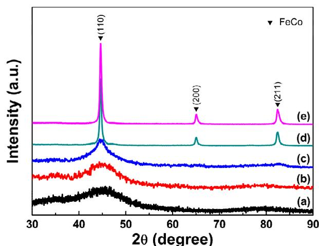
**Figure 5.** The XRD patterns of the original amorphous FeCo nanoparticles (a) prepared with 1.5 g PVP additions and the treated samples being annealed under Ar gas atmosphere at different temperature of 300 °C (b), 350 °C (c), 450 °C (d) and 550 °C (e) for 10 min.
