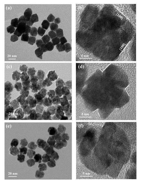
**Figure 3.** Morphologies of Pt–Pd nanostructures prepared at different temperatures. TEM images: (a) 170 °C, (c) 180 °C, (e) 190 °C; HRTEM images: (b) 170 °C, (d) 180 °C, (f) 190 °C.
