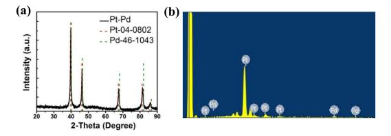
**Figure 2.** Composition analyses for the porous Pt–Pd nanoparticles synthesized at 190 °C: (a) XRD spectrum and (b) energy-dispersive spectroscopy (EDS) spectrum.
