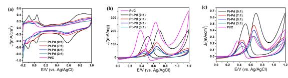
**Figure 6.** CV curves of Pt–Pd nanoparticles prepared by adding precursors with different ratios and commercial Pt/C: (a) in  $0.5 \text{ M H}_2\text{SO}_4$  solution; (b) in 1.0 M methanol +  $0.5 \text{ M H}_2\text{SO}_4$  solution, mass activities; (c) in 1.0 M methanol +  $0.5 \text{ M H}_2\text{SO}_4$  solution, specific activities. The scan rate was 50 mV/s.
