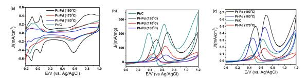
**Figure 5.** Cyclic voltammetry (CV) curves of Pt–Pd nanoparticles prepared at different temperatures and commercial Pt/C: (a) in  $0.5 \text{ M H}_2\text{SO}_4$  solution; (b) in 1.0 M methanol +  $0.5 \text{ M H}_2\text{SO}_4$  solution, mass activities; and (c) in 1.0 M methanol +  $0.5 \text{ M H}_2\text{SO}_4$  solution, specific activities. The scan rate was 50 mV/s.
