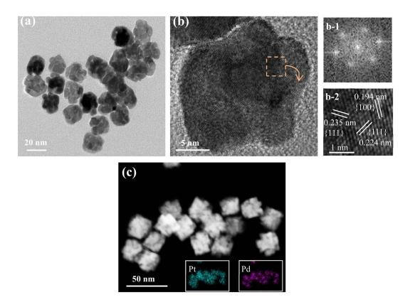
**Figure 1.** Morphology and composition analyses for the porous Pt–Pd nanoparticles synthesized at 190 °C: (a) Representative low-magnification TEM image, (b) high-magnification TEM image, (b-1) the corresponding Fourier transform (FFT) pattern, (b-2) the corresponding magnified TEM image, (c) high-angle annular dark-field scanning TEM (HADDF-STEM) image. The insets in (c) show the corresponding elemental mapping images of Pt (blue) and Pd (red) for porous Pt–Pd nanoparticles.
