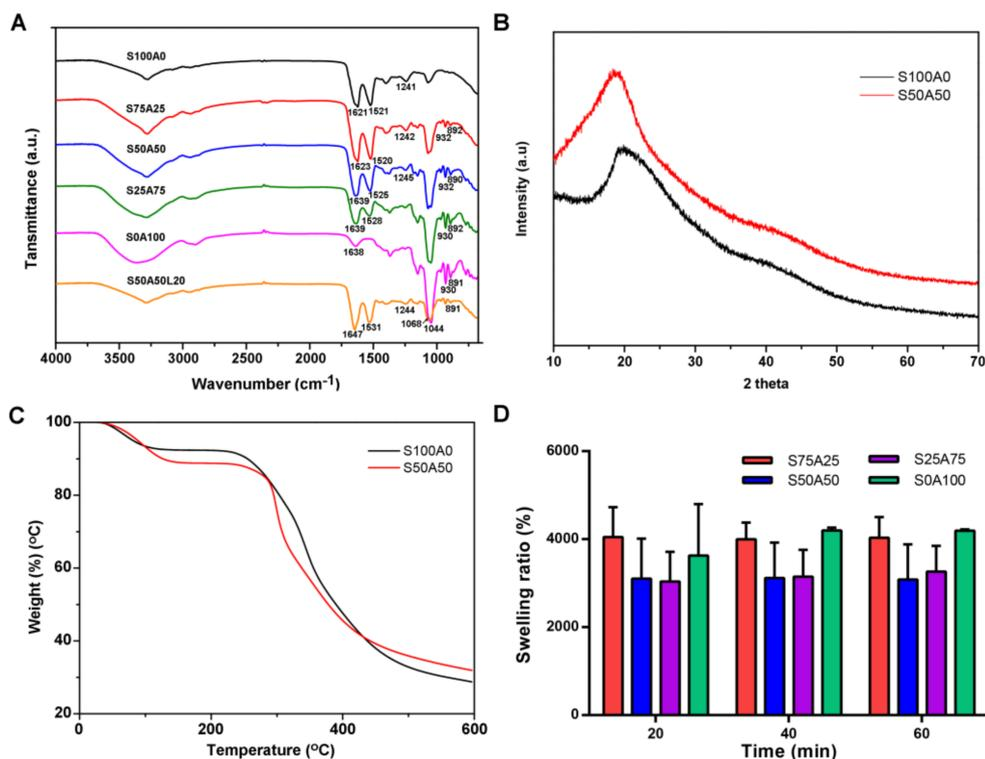
**Figure 3.** Characterizations of SS/AR gels. (A) Attenuated Total Reflection Fourier Transform Infrared Spectroscopy (ATR-FTIR); (B) X-Ray Diffraction (XRD); (C) Thermogravimetric Analysis (TGA); and (D) swelling ratio.
