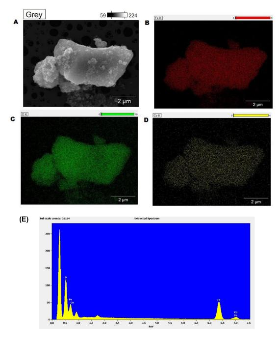
**Figure 3.** Elemental mapping (**A–D**) and energy dispersive X-ray spectrometry (EDX) analysis (**E**) of Fe<sub>3</sub>O<sub>4</sub>-Co<sub>3</sub>O<sub>4</sub> nanocatalysts.
