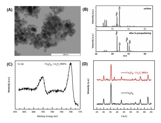
**Figure 2.** (**A**) TEM image of  $Fe_3O_4$ - $Co_3O_4$ ; (**B**) Positive mass spectra of  $Fe_3O_4$ -Co catalyst: (top) intact surface and (bottom) pre-sputtered surface; (**C**) Co 2p XPS line taken with the energy step of 0.1 eV and acquisition time window of 12 s; (**D**) PXRD spectra of  $Fe_3O_4$  (black) and  $Fe_3O_4$ - $Co_3O_4$ .
