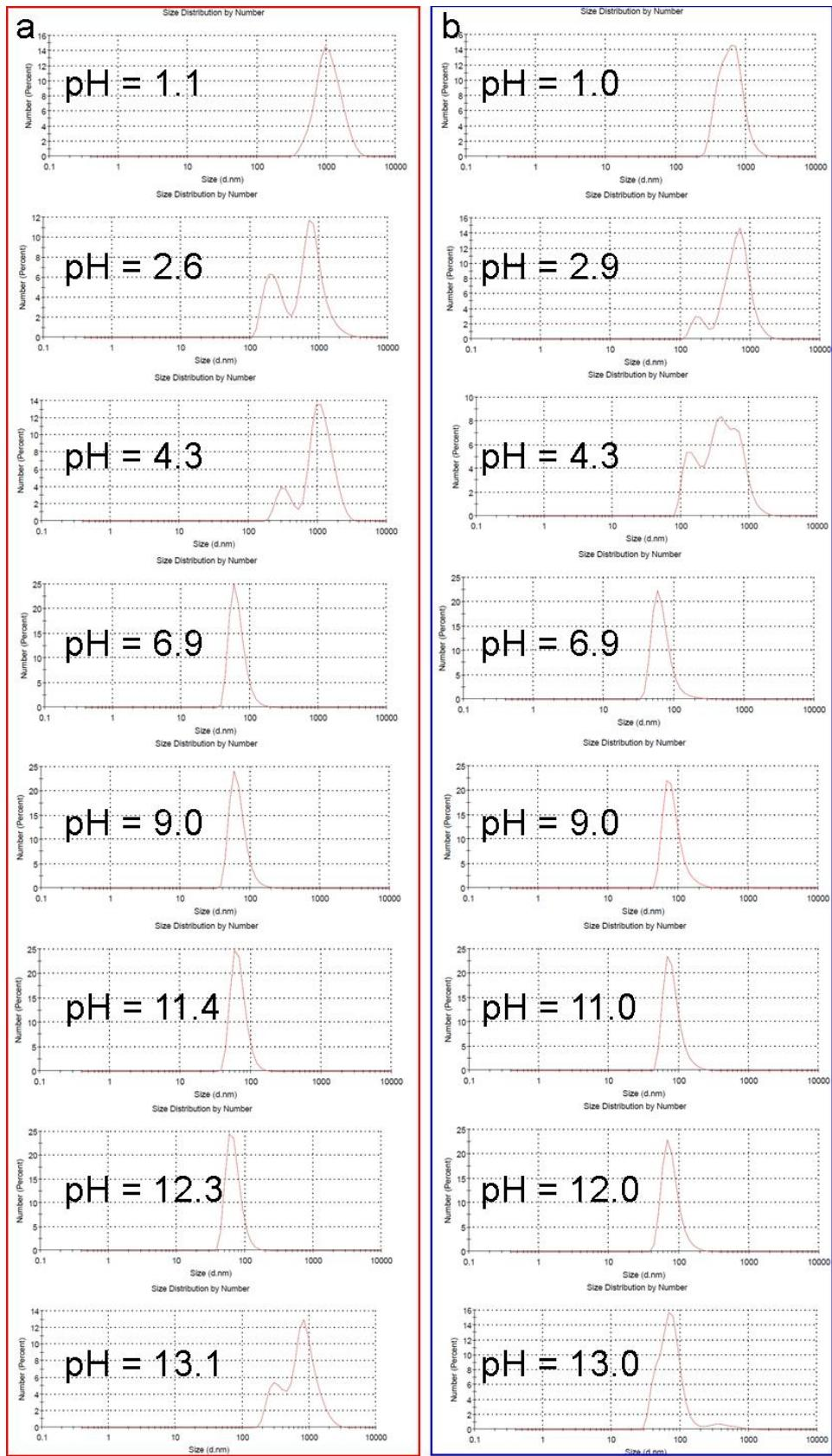
**Figure S4.** The size distribution of the 40 nm (a) and 85 (b) nm nanoclusters as a function of the colloidal solution pH variation, characterized by Dynamic Light Scattering (DLS) weighted by number.
