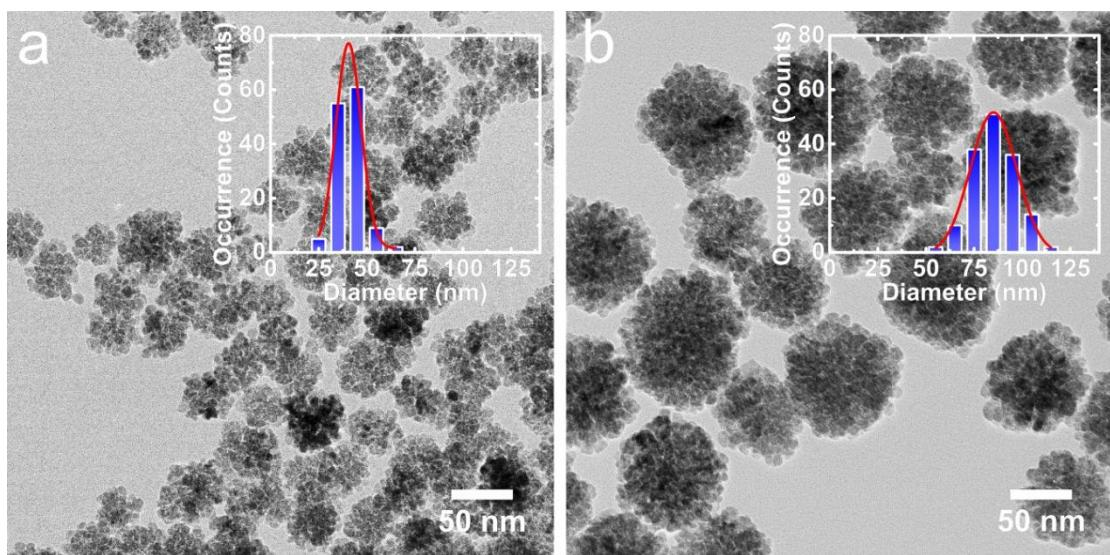
**Figure S3.** Low magnification TEM images and size distribution of specimens entailing 40 (a) and 85 (b) nm diameter nanoclusters.
