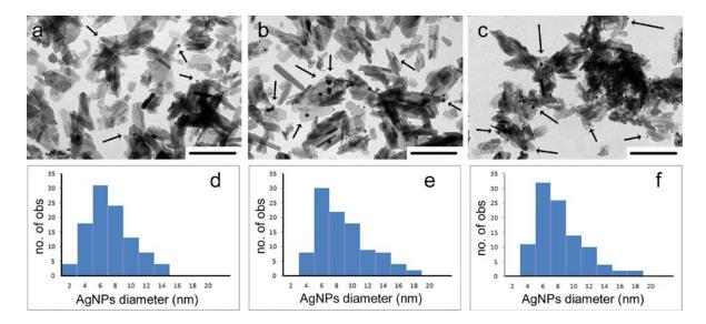
**Figure 2.** Transmission electron microscopy images of materials functionalized with AgNPs and related AgNPs size distribution diagrams: (**a**,**d**) HA-Ag50; (**b**,**e**) HSA10-Ag50 and (**c**,**f**) HSA20-Ag50. The arrows in micrographs indicate AgNPs. Bars = 200 nm.
