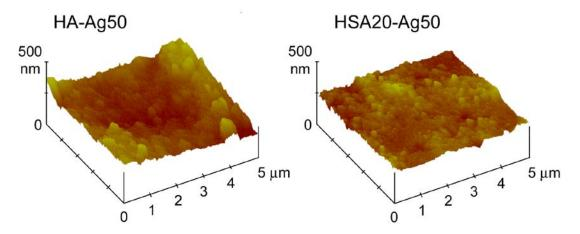
**Figure 5.** Atomic force microscopy images of the surfaces of disk-shaped samples obtained by pressing as-prepared HA-Ag50 and HSA20-Ag50 powders into cylindrical molds.
