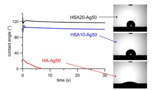
**Figure 4.** Plots of contact angle values as a function of time. The images of droplets measured after 1 second on different composite materials are shown on the right.
