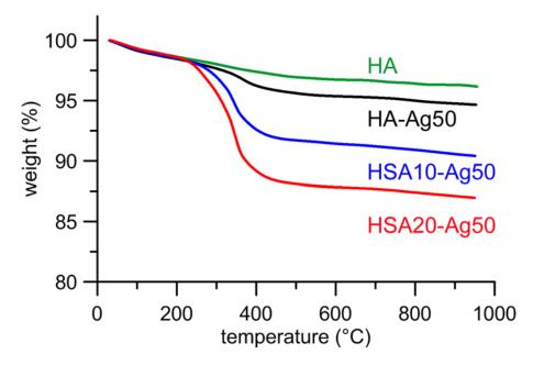
**Figure 3.** Thermogravimetric plots of as-prepared HA, HA-Ag50, HSA10-Ag50, and HSA20-Ag50, useful for quantification of HSA in the composite materials.
