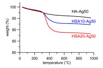
**Figure 7.** Thermogravimetric plots of HA-Ag50, HSA10-Ag50, and HSA20-Ag50 after 14 days soaking in DMEM.
