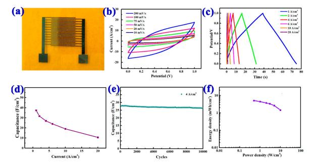
**Figure 3.** (a) Photos of the MSC devices; (b) capacitance-voltage (CV) curves at various scan rates; (c) Galvanostatic charge-discharge (GCD) at different currents measured in the voltage window of 0-1 V; (d) comparison of capacitances of the MSC devices at varied galvanostatic charge-discharge current densities; (e) capacitance retention on cycle number at a current of 4 A/cm<sup>3</sup>; (f) energy and powder densities of the MSC devices.
