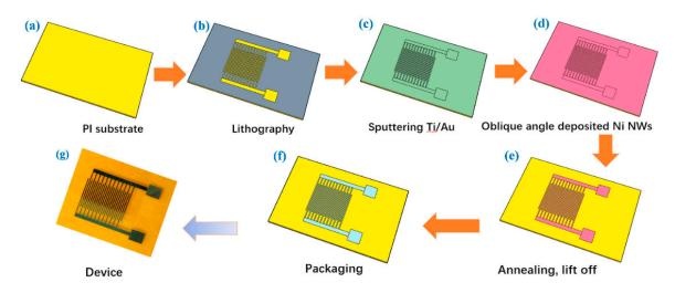
**Figure 1.** The schematic fabrication process of flexible micro-supercapacitors (MSCs). (**a**–**f**) Steps of preparing substrate, lithography, sputtering Ti/Au, oblique angle-depositing Ni nanowires annealing and packaging, respectively; (**g**) photograph of the as-fabricated flexible supercapacitor device.
