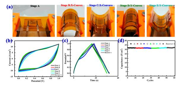
**Figure 4.** (a) Photos of a MSC at different bending states; (b) CV curves at 100 mV/s in straight and different bending states, respectively; (c) charge/discharge curves at a current of 2 A/cm<sup>3</sup> in straight and different bending states, respectively; (d) capacitance performance under the different bending states.
