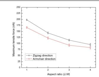
Figure 3. Tensile loading characteristics of single layer BNNS of varying aspect ratios at 300 K.
