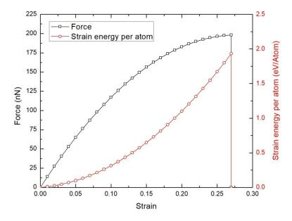
Figure 2. Force and strain energy graph of BNNS under tensile loading at 300 K.
