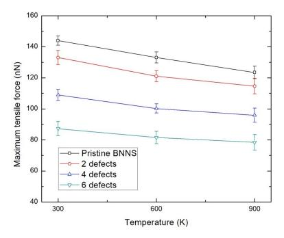
Figure 6. Tensile loading characteristics of BNNS at various temperatures with vacancy defects.
