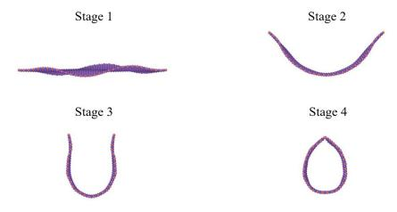
Figure 7. Stages of bending in BNNS to form a BNNT.
