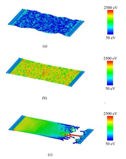
**Figure 4.** Tensile loading stages of single-layer BNNS at 300 K at (a)  $\varepsilon = 0.0$ ; (b)  $\varepsilon = 0.12$ ; and (c)  $\varepsilon = 0.25$ .
