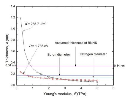
**Figure 8.** Determination of the correct thickness and Young's modulus of BNNS from the intersection of axial stiffness and bending stiffness curves on the *E*-*h* coordinate plane.
