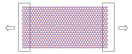
**Figure 1.** Simulation of BNNS under tensile loading. The atoms enclosed inside the black rectangle at either ends of BNNS is subjected to tensile loading. The loading direction is indicated by the arrows. Atoms depicted in ochre are boron and atoms depicted in blue are nitrogen.
