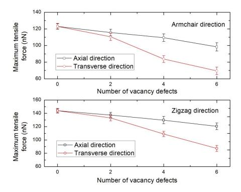
**Figure 5.** Tensile loading characteristics of single layer BNNS with vacancy defects along the axial and transverse directions at 300 K.
