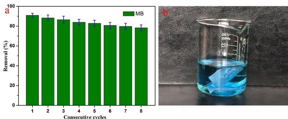
**Figure 10.** Relative adsorption reutilization studies towards removal of MB for different consecutive cycles at room temperature of PCL/(50%)PCD composites (a) and the photograph of PCL/(50%)PCD composite after eight reutilization cycles (b).
