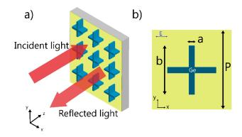
**Figure 1.** Perspective views of the hybrid metasurface absorber (**a**) and the unit cell (**b**). The height of the resonator is constant at  $h = 0.95 \mu$ m; the period p and geometric parameters a and b vary for different resonance wavelengths.
