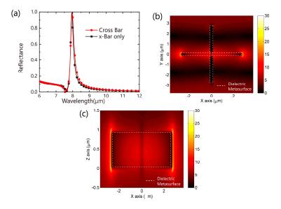
**Figure 2.** (a) The reflectance spectra of the dielectric metasurfaces (cross bar and *x*-bar only) without metal film., A Fano resonance is observed with the full-width at half-maximum (FWHM) 220 nm. The E-field distribution of the metasurface in *x*-*y* plane (b) and *x*-*z* plane (c) at 7.98  $\mu$ m. There is a strong E-field localization at the ends of the horizontal bar.
